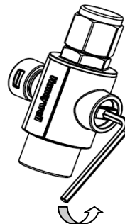
Fig. 7. Turn anticlockwise to open the exhaust valve
