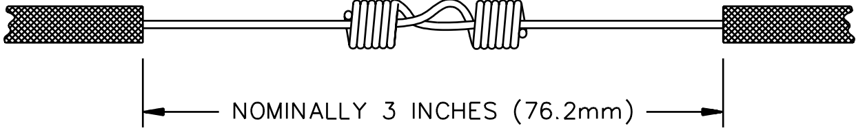
Figure 13.1 Western union splice
