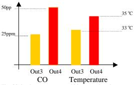
The CO level or temperature, whichever reaches the preset trip point activates the relay contacts. 25ppm CO or 33  $^{\circ}$ C in temperature will trigger relay contact at Out3; while 50ppm CO or 35  $^{\circ}$ C temperature will trigger second relay contact at Out4.
