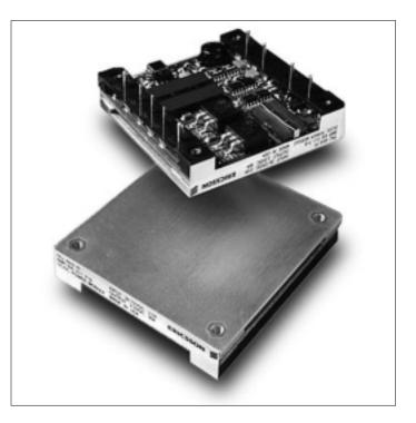
The PKJ 4000B series represents another one of Ericsson's "industry first" achievements in the continued development of our "Third Generation" of high-density, high-efficiency power modules. This module packs 57.9 W/in<sup>3</sup> at 89% efficiencies (3.3V @ 40A) in an industry standard half-brick package. These breakthrough features come from using the most advanced patented topology utilizing integrated magnetics and synchronous rectification on a low-resistivity multilayer PCB.
