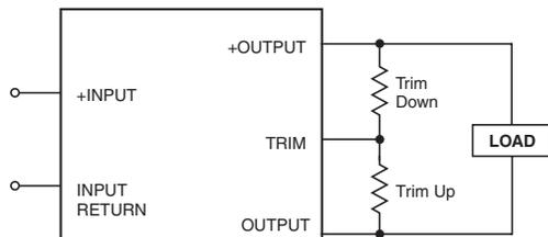
**Note:** Install either a fixed trim-up resistor or a fixed trim-down resistor depending upon desired output voltage.
