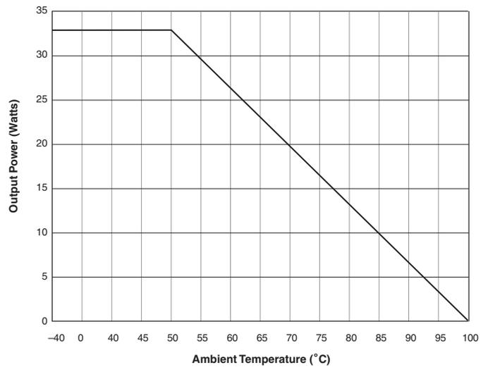
UNR-3.3/8-D5T/D5SM Output Power vs. Ambient Temperature, No Air Flow
