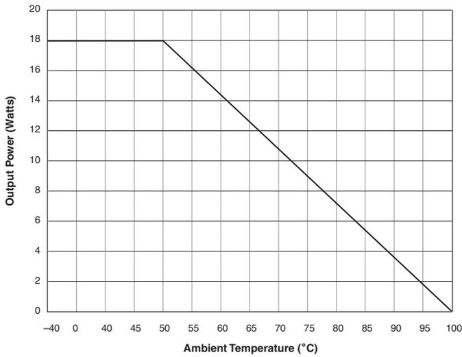
UNR-3.3/8-D12T/D12SM Output Power vs. Ambient Temperature, No Air Flow
