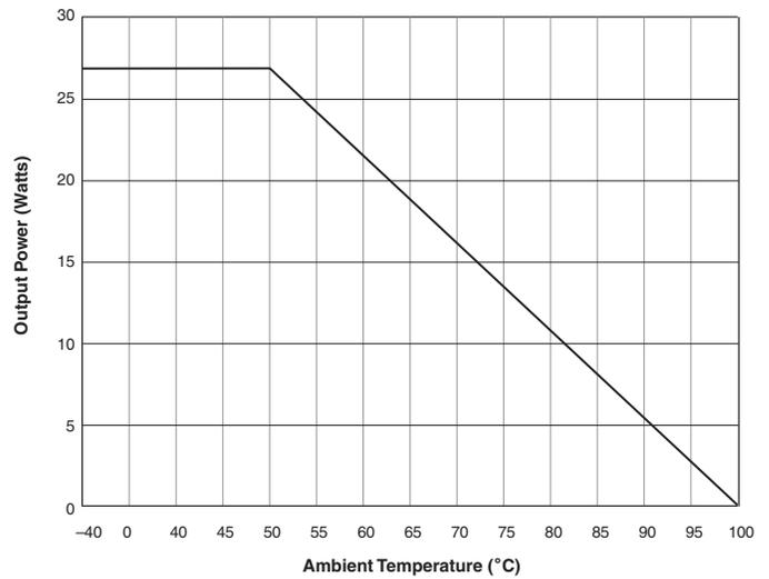
UNR-2.5/10-D5T/D5SM Output Power vs. Ambient Temperature, No Air Flow
