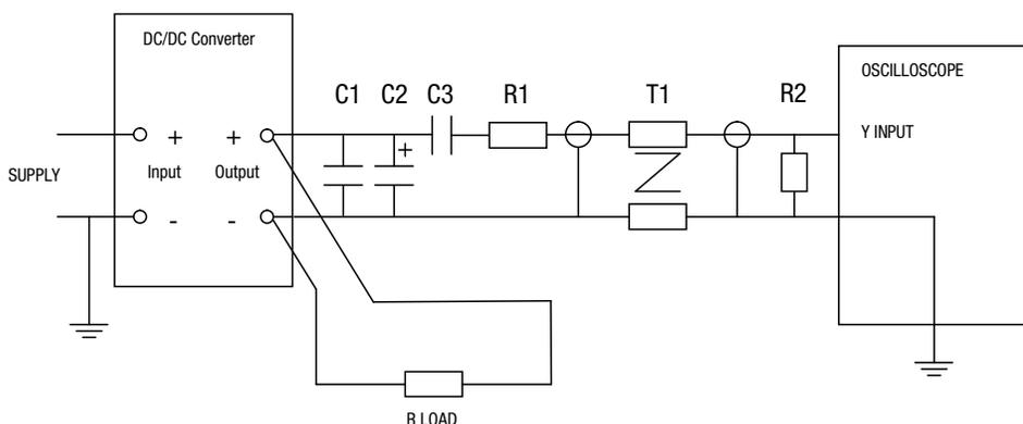
**Input Reflected Ripple Current Test Method**
