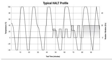
changes, stresses are stepped up again and the cycle is repeated until the "fundamental limit of the technology" is determined.
