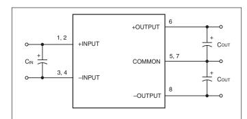
Figure 2. Using External Capacitors to Reduce Input/Output Ripple/Noise
