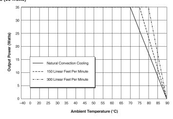
Figure 4a. Temperature Derating Without Heat Sink
