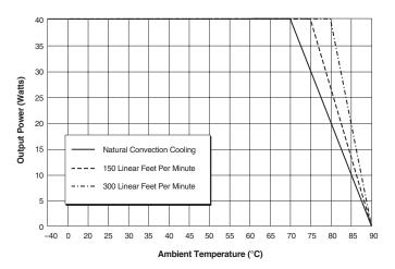
Figure 5b. Temperature Derating With Heat Sink
