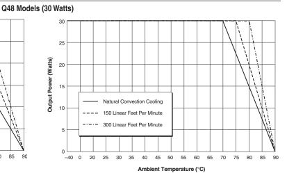
Figure 3a. Temperature Derating Without Heat Sink
