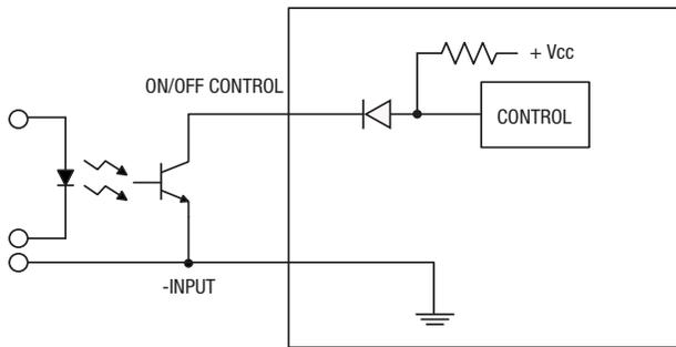
**Figure 4. Driving the Positive Polarity On/Off Control Pin**
