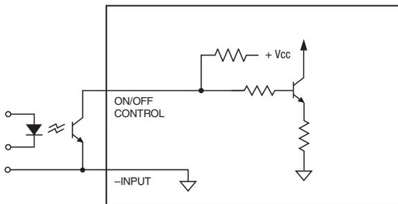
**Figure 5. Driving the Negative Polarity On/Off Control Pin**
