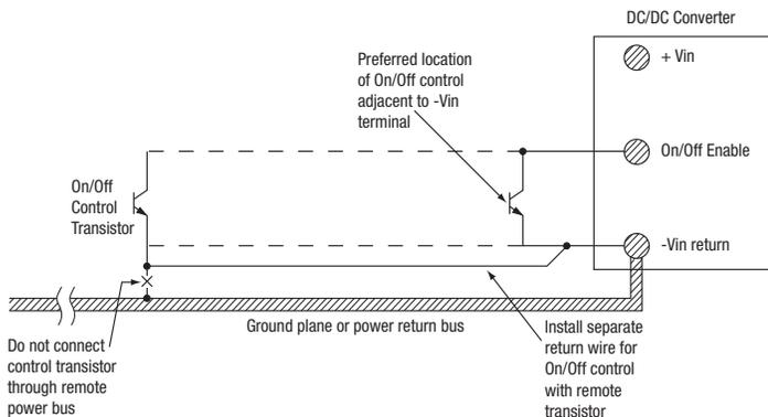
**Figure 9. On/Off Enable Control Ground Bounce Protection**
