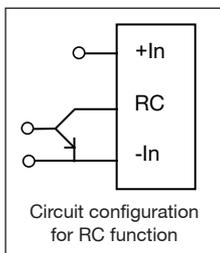
The PKJ 4000E Series DC/DC converters have a remote control function referenced to the primary side (- In), with negative and positive logic options available. The RC function allows the converter to be turned on/off by an external device like a semiconductor or mechanical switch. The RC pin has an internal
