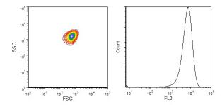
**Figure 2.** FSC-SSC plot and fluorescence histogram in the PE/Texas Red channel of Zepto<sup>TM</sup> Ultra Orange Carboxyl Microspheres on a flow cytometer.
