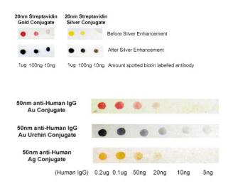
Figure 1. Example dot-blot assay for Cytodiagnostics streptavidin gold conjugate (top left) and our streptavidin silver conjugate (top right) before and after enhancement using Cytodiagnostics silver enhancement kit for membranes. Bottom picture illustrates and highlights the difference in appearance (color) of 50nm anti-human IgG noble metal nanoparticle conjugates prepared using NHS-activated gold nanoparticles, NHS-activated gold nanoparticles, and NHS-activated silver nanoparticles,
