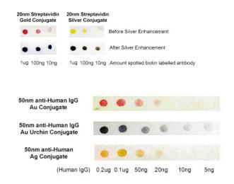
Figure 1. Example dot-blot assay for Cytodiagnostics streptavidin gold conjugate (top left) and our streptavidin silver conjugate (top right) before and after enhancement using Cytodiagnostics silver enhancement kit for membranes. Bottom picture illustrates and highlights the difference in appearance (color) of 50nm anti-human IgG noble metal nanoparticle conjugates prepared using NHS-activated gold nanoparticles, NHS-activated gold nanoparticles, and NHS-activated silver nanoparticles,
