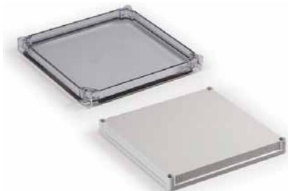
The enclosure cover can be transparent so that the status of the equipment inside is easy to monitor. In thermoplastic enclosures, the whole cover is either grey or transparent. Grey covers are available both in ABS and polycarbonate. Transparent covers are available only in polycarbonate.
