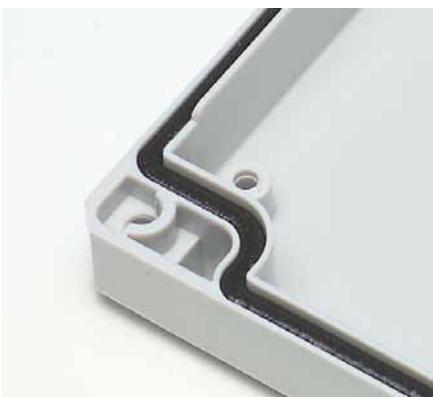
We use injected, jointless PUR (polyurethane) gaskets in our thermoplastic and steel enclosures to ensure a high protection class. The standard gasket material of our aluminum and polyester enclosures is neoprene. Some enclosures are available with a silicone gasket, on request.
