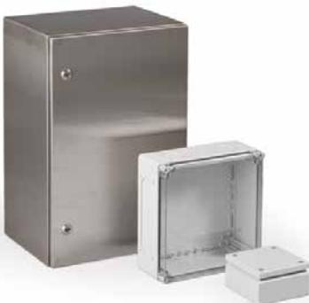
Our Ensto Cubo range includes enclosures made of thermoplastics (ABS and polycarbonate), polyester, sheet steel (polyester painted mild steel and stainless steel, AISI 304 or AISI 316) and aluminium. We use high quality materials provided to us by the world's leading suppliers. The right
