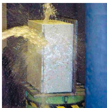
Provided by enclosures, the degree of protection is an important factor. The degree of protection is defined purely for the enclosure and should be maintained during the installation work, meaning that, for instance the IP class of the cable glands used for cable entries should be higher or the same as that of the enclosure.
