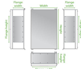
The flange openings are either only on the base of the enclosure, or on both sides and the base.
