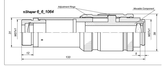
Figure 5. Flat Top Beam Shaper basic mechanical design.
