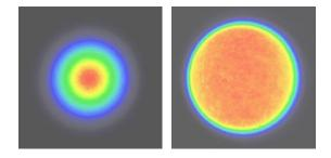
Angular magnification of the telescopic system is about 0.65. Thus, from the point of view of paraxial optics, the diameter of the output beam is increased by factor 1/0.65 while the field angle is reduced by a factor 0.65.
