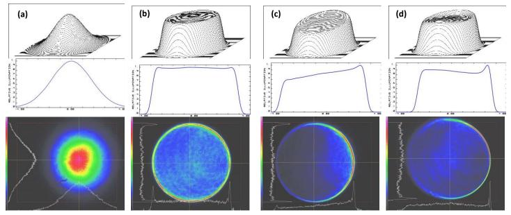
Figure 12 To evaluation of sensitivity of misalignments, theoretical and experimental intensity profiles for Flat Top Beam Shaper 6\_6\_1064 @ 1064nm:
