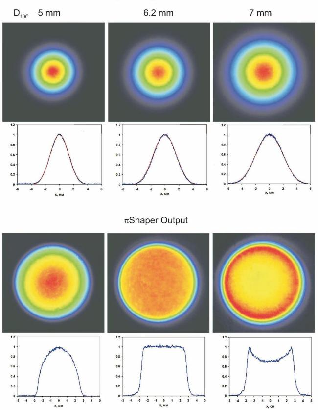
Figure 10. Flat Top Beam Shaper operation by variable diameter of perfect Gaussian input beam.
