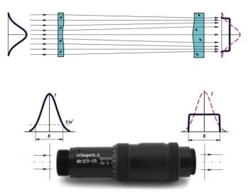
Figure 1. Refractive field mapping beam shaper Flat Top Beam Shaper.
