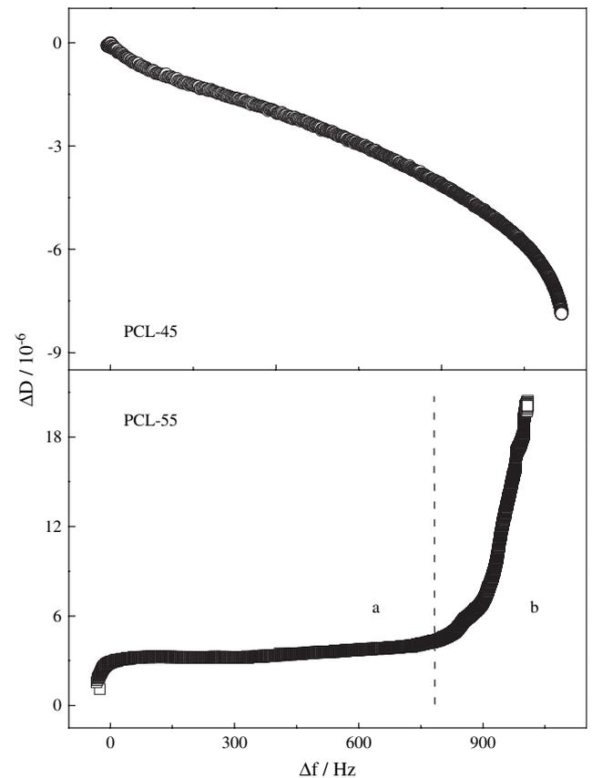
Fig. 4. The relations of  $\Delta D$  vs  $\Delta f$  for enzymatic degradation of PCL-45 and PCL-55 catalyzed by lipase PS at  $n = 3$ , where  $C_e = 0.5$  mg/mL.
