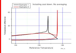
the data against temperature. This is shown below. Consider the lower lines in the plots (these represent heating—the upper lines are from cooling). The aged
