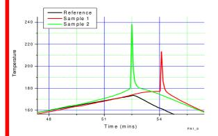
A zoom of the data before the ignition is very revealing. The fresh sample (Sample 1) follows the reference temperature whilst the aged sample (Sample 2) shows exothermic deviation and ignition prior to ignition of the fresh sample. There is a clear difference in stability.
