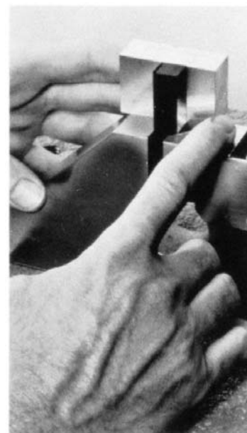
FIG. 4 Jig for Positioning Specimen for Clamping
