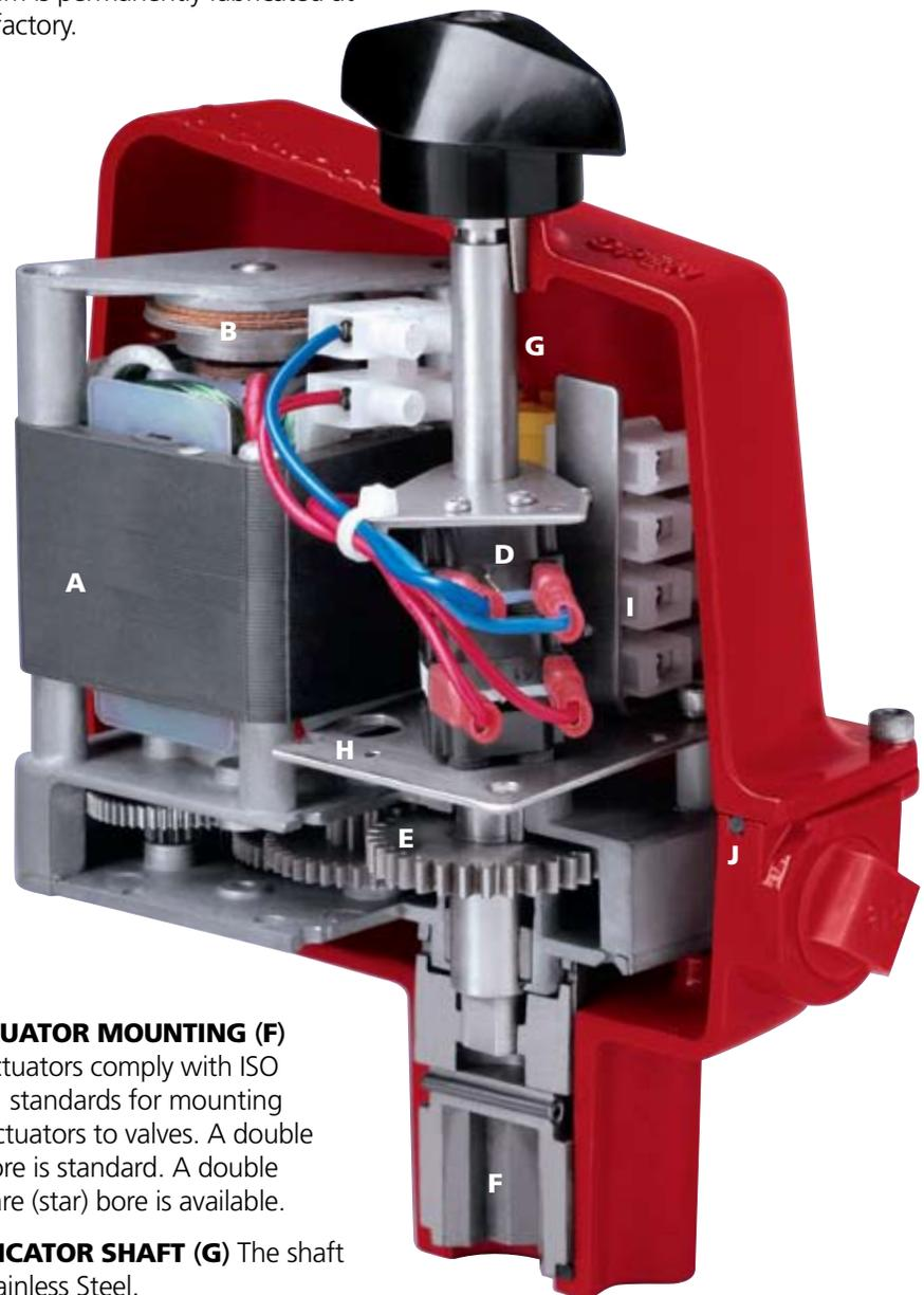
**ACTUATOR MOUNTING (F)** R<sup>5</sup> actuators comply with ISO 5211 standards for mounting of actuators to valves. A double D bore is standard. A double square (star) bore is available.
