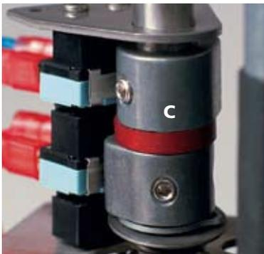
**TRAVEL LIMIT SWITCHES (D)** Bray has provided two SPDT switches as standard. The 10A, 220 VAC switches are used for AC motor control. Two optional auxiliary switches are available to signal a low wattage AC lamp or a DC controller input. Switches are easily accessible without interference from other components.
