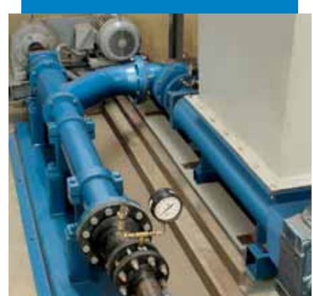
The Moyno 2000 HS system is a significant technology advancement for the wastewater treatment industry. It can pump filter cake further distances with higher volumetric efficiencies than any other progressing cavity pump.
