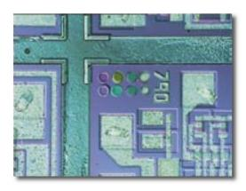
• Semi-conductor, DIC, 20x Plan Fluor, video adapter with 0.4x.
