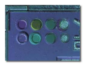
• Semi-conductor, DIC, 20x Plan Fluor, video adapter with 1.2x.
