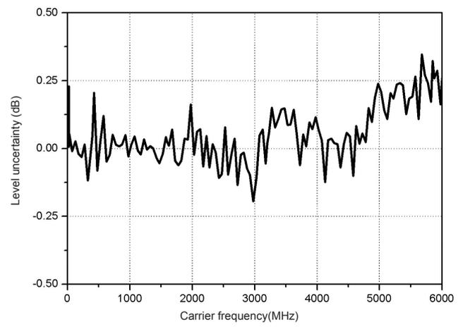
Measured -127dBm output level VS frequency
