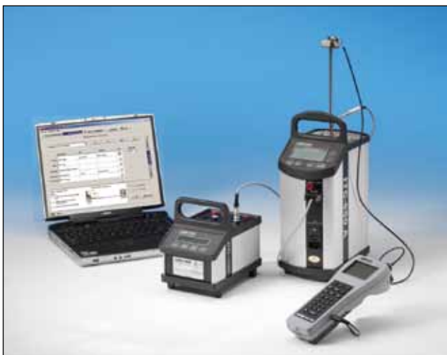
Set-up with JOFRA ASC300, ITC temperature calibrator and DTI-1000 reference thermometer connected to a PC with JOFRACAL
