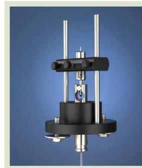
This heavy-duty swivel holder bolts to the top of the cage and allows all of Instech's single and dual channel swivels to be used with dogs, nonhuman primates and other large animals. For cleaning, simply remove the swivel and the stainless steel posts and send the rest of it through a cage washer with the cage. The mount couples directly to standard 1/2-in (12.7mm) ID jacket tethers.
