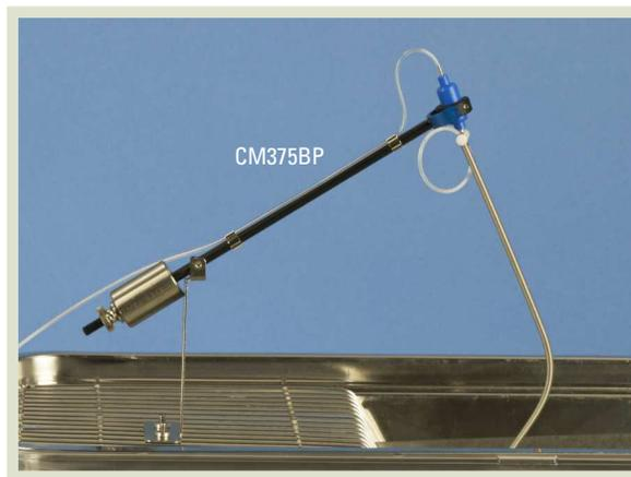
This mount is designed for standard infusion of rats in shoebox cages. The mount pivots in the vertical plane to remove slack from the tether but allow enough length to reach all corners of an asymmetrical cage. The adjustable counter-weight can be set to balance the weight of our swivels plus a tether. The crossbar in the wire top must be clipped in the slot that the tether is placed for maximum travel.
