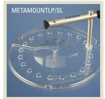
These mounts hold a swivel in a fixed position above a standard Techniplast (Nalgene) or Lab Products metabolism cage. Parts included: vertical and horizontal mounting bars with hardware, new cage top with pre-drilled mounting holes. Available with slotted lids for easier access to the animal.
