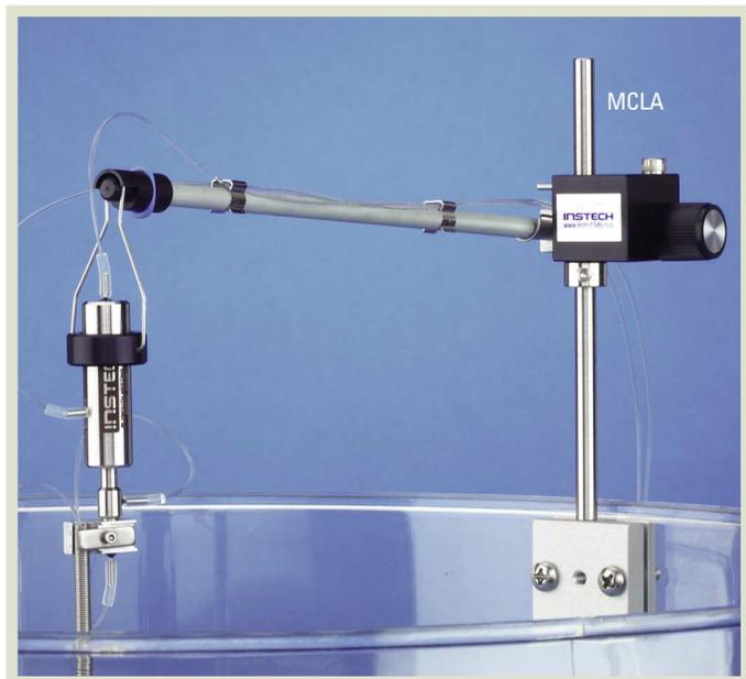
These counter-balanced lever arms move vertically and horizontally with the animal to prevent slack in the tether. Their sensitivity makes them ideal for awake-animal microdialysis and all types of infusion studies with mice. They feature an adjustable spring counter-balance, not a mass, which increases their responsiveness to an animal's quick movements.
