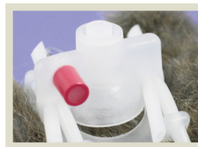
VAH95AB-1P harness with side port for intermittent manual dosing or sampling
