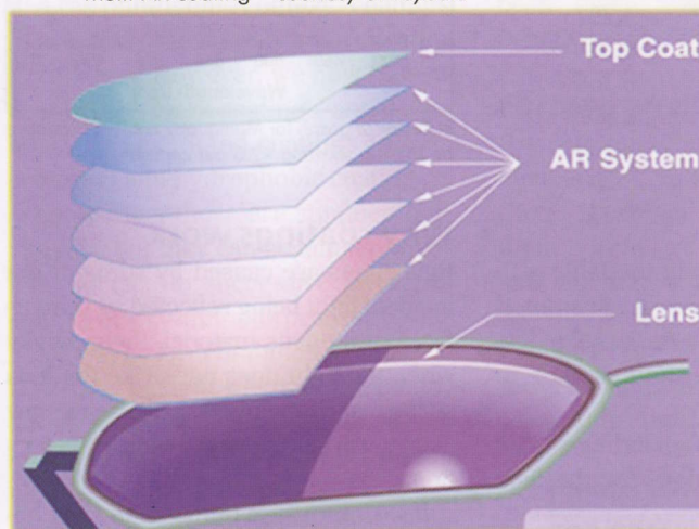
Fig. 2: A schematic showing the structure of a typical high quality multi-AR coating – courtesy of Leybold
