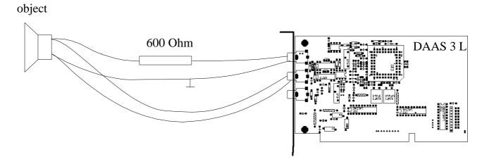
Connect the input "Line" directly to the object as shown to avoid measuring the cable! Now start with the actual measurement.
