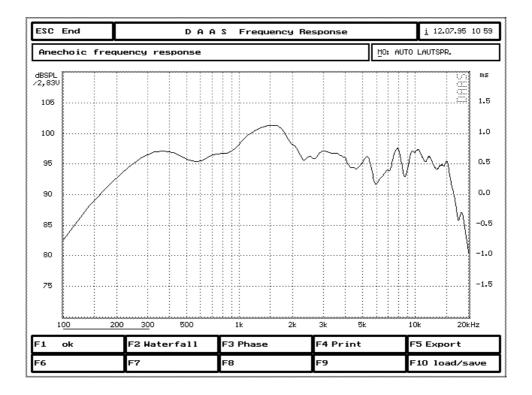
The curve can be saved using [F10] = "load/save" and re-loaded at a later date. A corrected phase response is also available under [F3].
