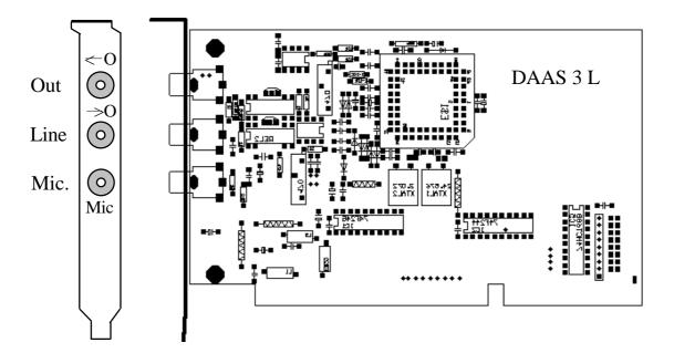
The DAAS card has 2 inputs and one signal output. The microphone is connected to the "Mic" socket. Using the microphone supplied the maximum sound pressure is  $\pm 2$  Pa and  $\pm 8$  Pa.
