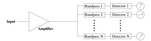
When the middle frequencies are so chosen that the filter bands border exactly with each other a complete spectrum can be achieved. With this system the entire frequency response curve can be obtained with only two individual measurements.
