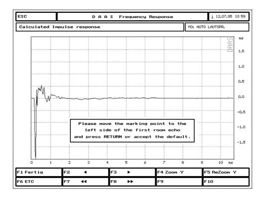
Note that cutting out the echoes reduces the frequency resolution. The resolution is a result of 1/measuring time. If the marker is position at 5 milliseconds the resolution will be 200 Hz.
