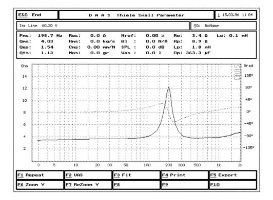
Hint: Except for tweeters it is recommended to use the sample rate 6 kHz (default). Measuring a bass speaker it is recommended to use resistors between 100 and 470 ohms.
