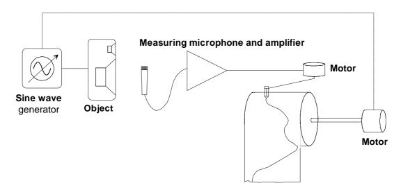
By the use of a plotter as shown above a continuous response curve can be obtained. If a bandpass filter, the middle frequency of which can be changed in synchronization with the generators frequency, is inserted between microphone and plotter, it is possible, within certain limits to remove room reflections, i.e. it is possible to achieve free field measurements within a sealed room. This principal is known by the name "TDS".
