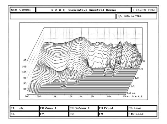
Here too the time axis can altered with Zoom In t and Zoom Out t. However by using the zoom function all the curves are recalculated. The default setting for the time axis can be changed.
