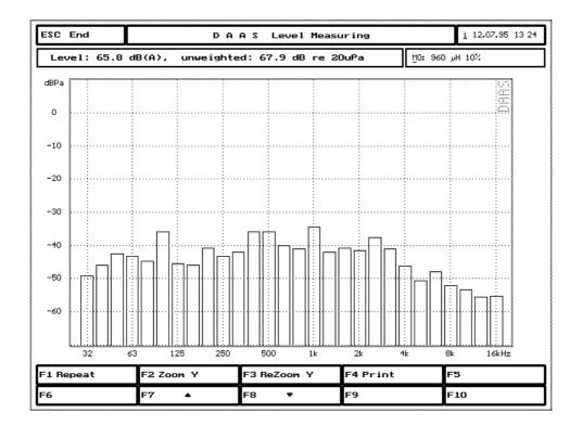
To measure the signal to noise ratio of an amplifier, feed the input with a sine wave (say 1kHz) and measure the level on the output. (20 V range, load resistor on output!). Increase the volume setting and repeat the measurement until the output voltage is just about to be limited. Note the level. Switch the input signal off and measure the amplifier noise in the 0,2 V range. The difference between the two levels is the signal to noise ratio, A-weighted and without weighting.
