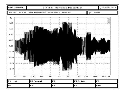
The signal tones are combined to form a single picture. Left are the low frequencies and right the highest. Press [F1] to calculate the harmonic distortion curve:-
