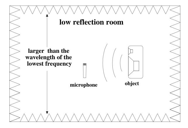
For a measurement down to 50 Hz the minimum size is 6,8 Meter (!) nett. The absorbent wedges must be 0,25 \* wavelength i.e. 1.7m. This gives a total of around 10m!!!
