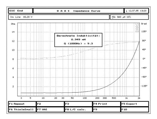
The range for inductance is approx.  $6 \mu H$  to about 10 mH and for capacitance approx.  $1 \mu F$  to  $100 \mu F$ . For larger values the sample rate must be reduced.
