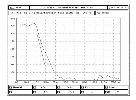
Shift this line using [F2] / [F3] and [F7] / [F8] until itis identical with the slope of the acoustic level curve. Smooth the acoustic level curve using [F5] if necessary.
