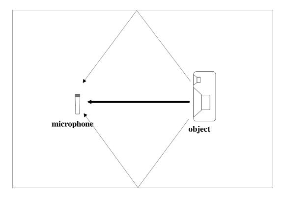
The undesirable reflections can be removed with the function [F2] "free field frequency curve calculation"
