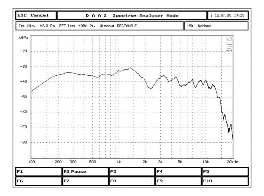
For this frequency response measurement the smoothing option mentioned above is very useful. Set the smoothing option to 'yes' to get a soft curve, or set the smoothing option to 'Terz' to get octave/3 bars.
