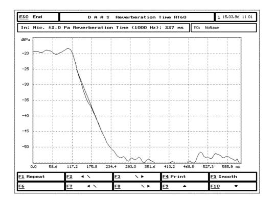
In the info line on the top of the screen now the reverberation time is shown. Note that smoothing the acoustic level curve will increase the lowest measurable reverberation time.
