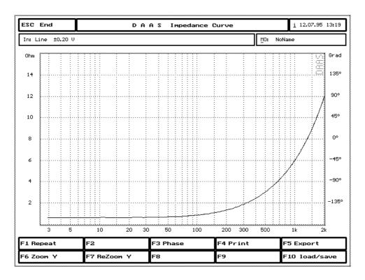
Using [F6] and [F7] the scaling can be changed from 1 Ohm/Div to 32 Ohm/Div. Press [F3] to calculate and show the phase curve.
