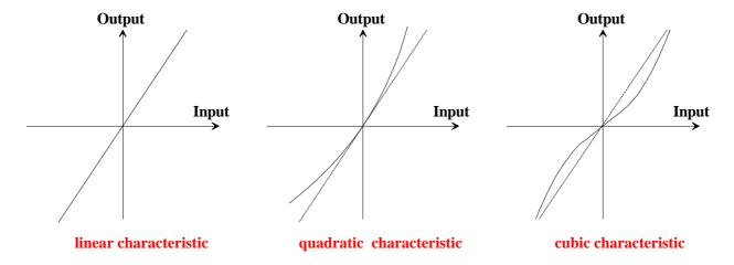
Generally gain characteristics are made up of elements of linear, quadratic and cubic characteristics.
