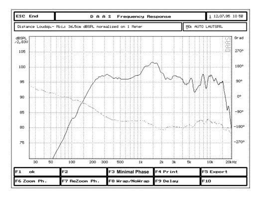
If the option 'Wrap/NoWrap' is activated (key [F8]), the phase response curve will be wrapped at  $\pm 180^{\circ}$ .
