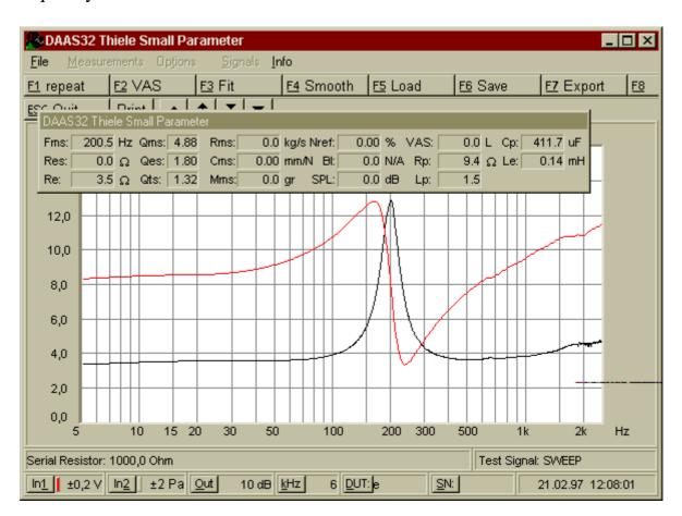
Use 'Load' and 'Save' like described in chapter "Impedance measurement". Use the 'Smooth' function cautious, because the impedance maximum peak will be reduced.
