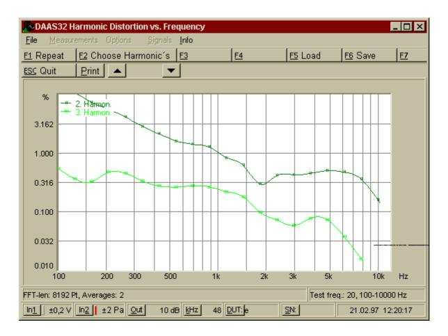
Press or click <u>F2</u> Choose Harmonics" to select the visible harmonic components. Use F5 and F6 to save and load distortion curves.
