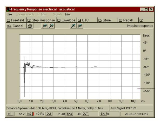
Press F2 to get the step response. The step response is the sound pressure level response a loudspeaker produces when driven by an on-switched direct-current-level.
