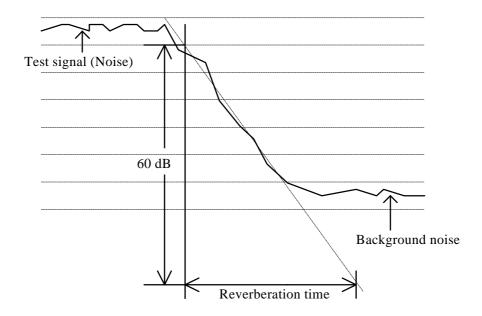
But the disadvantage of this method is that the reverberation time usually dependst on the frequency. Harmonic signals for supplying the speaker are not usable, because stationary acoustic waves will falsify the results. The DAAS®32 uses narrow band noise with variable center frequency to avoid this disadvantages. This method is very easy to use and don't need complex parameters to set.
