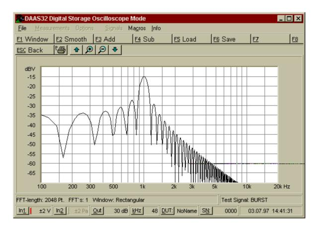
With F1 the weighting window is selected. Use F2 to smooth the curve. Use the Zoom keys and the arrow keys to adjust the display range.
