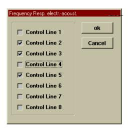
In this example the control lines 2,3 and 5 are activated if you are measuring an electrical - acoustical frequency response.
