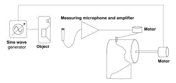
By using a plotter as shown above a continuous response curve can be obtained. If a bandpass filter, the middle frequency of which can be changed in synchronization with the generators frequency, is inserted between microphone and plotter, it is possible, within certain limits to remove room reflections, i.e. it is possible to achieve free field measurements within a sealed room. This principle is known by the name "TDS".
