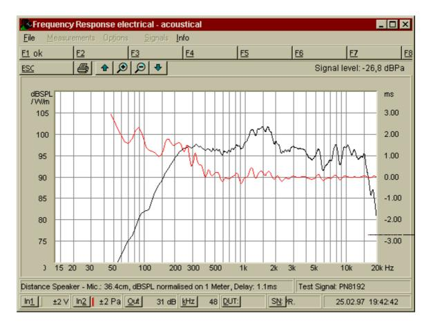
is the deviation from the via automatic delay compensation determined group delay.
