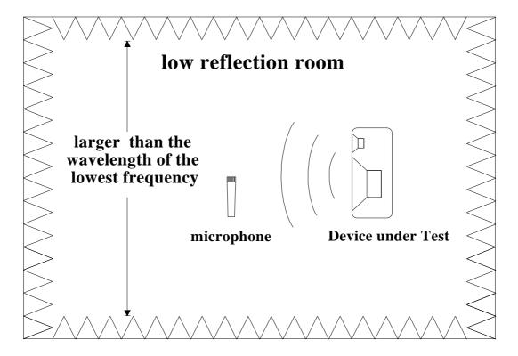
For a measurement down to 50 Hz the minimum size is 6,8 meter (!) net. The absorbent wedges must be 0.25 \* wavelength i.e. 1.7 m. This gives a total of around 10 m !!!
