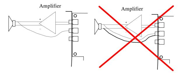
A connection between the input ground and the output ground of a hi-fi amplifier may result a high frequency oscillation with a high amplitude. This may damage your amplifier!
