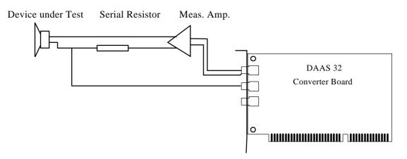
All connections should be very short and should have low impedance to avoid measuring errors. The cable to the input 'Line' should be connected close to the Device under Test.
