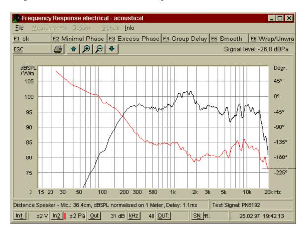
The phase will be unwrapped shown. This means if the phase curve will achieve e.g. 180° it will not jump to -180°. You can change this option using F6.
