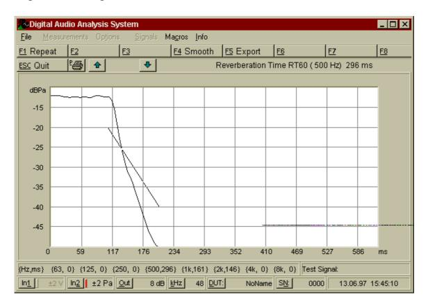
Shift this line until the slope of this line is identical with the slope of the acoustic level curve. To shift this line move the mouse to the upper end or to the lower end of the line, then press the left mouse button and move the chosen line end.
