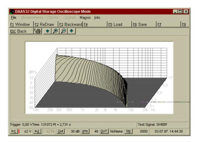
The waterfall diagram can also be rotated. Use "F3 Backward" to get the rotated waterfall diagram.
