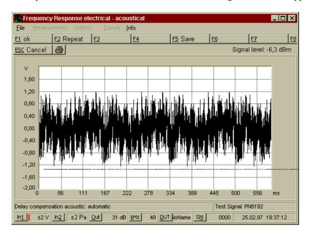
If the signal is too large a warning beep will be audible, and if it is too small a warning message will appear. If you ignore these warnings, the measurement accuracy will be reduced. In both cases the amplifier volume control or the input sensitivity should be adjusted and the operation repeated.
