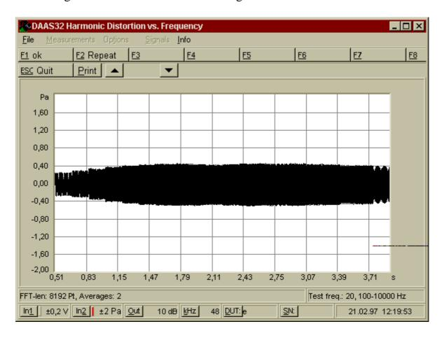
The signal tones are combined to form a single picture. Left are the low frequencies and right the highest. Press F1 to calculate the harmonic distortion curve:
