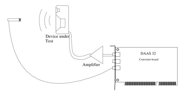
The spectrum now shown is directly the frequency response curve of the object (speaker). Note that the curve shown is a relative curve, the absolute values (e.g. 2 Pa/V) cannot be read directly from here.
