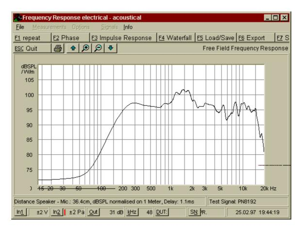
The area which is likely to be of little use due to the reduced frequency resolution is marked by a line on the frequency axis scale.
