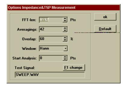
WARNING The options for impedance curve and Thiele Small parameter measurements form a vital part of the evaluation algorithms. Changes may well have a negative effect on system performance (increase in evaluation time, false results and large errors)! All settings are optimized by the manufacturer and should only be changed for special applications and only by persons who are fully familiar with the techniques of digital signal evaluation.
