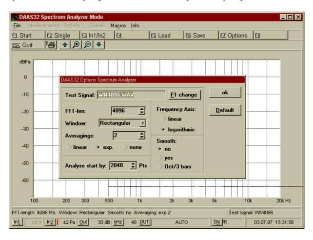
Choose the test signal using F1. The FFT length (number of points) can be changed in the range 512 points to 65536 points. The FFT length in conjunction with the sampling rate will designate the frequency resolution:
