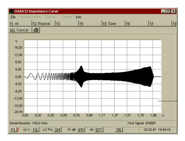
As a rule the input range is 2 V. Except by using serial resistors greater than 1000  $\Omega$  or measure very low impedance values the input range should be set to 0.2 V.
