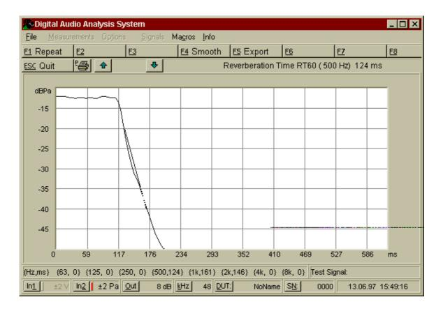
On the top of the screen in the info line now the reverberation time is shown. Additional all measured values since start of RT 60 measurement are shown in the status line. You can write this values to a text file by using the "Export" function.
