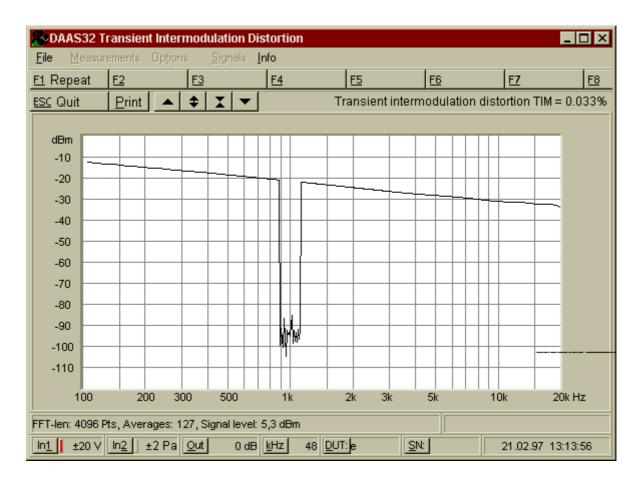
The level in this removed octave/3 band will be measured and related to the level in this band without removing.
