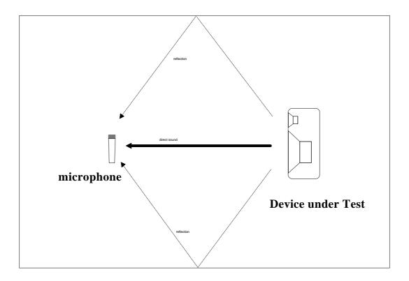
The undesirable reflections can be removed by using the impulse response. In the waveform of the impulse response it is possible to see the echoes resp. the reflections. Search in the area of 3 to 10 milliseconds for a copy of the main impulse of the signal which appears between 0 and 1 milliseconds. For better detection of echoes you can change the display range using the
