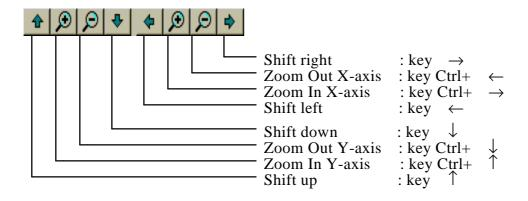
The lower section of the DAAS<sup>®</sup>32 window contains the status line and various control buttons. In the status line there are some actual measurement parameters shown such as FFT length, weighting window, averagings, test signal and so on. With the control buttons there are the following adjustments possible:
