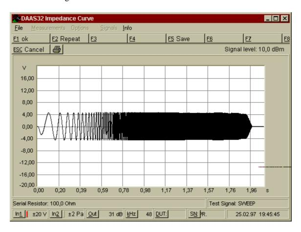
If something is wrong, check the connections or change the measurement level and repeat the reference measurement.
