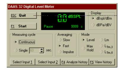
The measuring time can be set by using the "single" switch. On "Continuos", the measurement cycle will go on until the ESC key is pressed.
