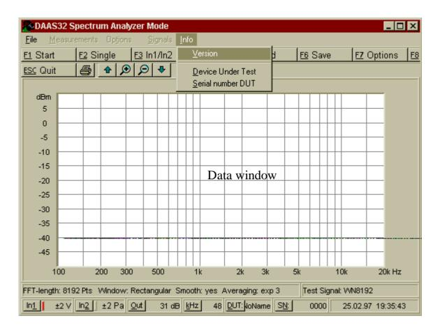
At the top of the window below the title bar you will find the menu bar. Here you can start the various measurements, setup the options, start the signal player and recorder, get the version info and enter the Device under Test infos.
