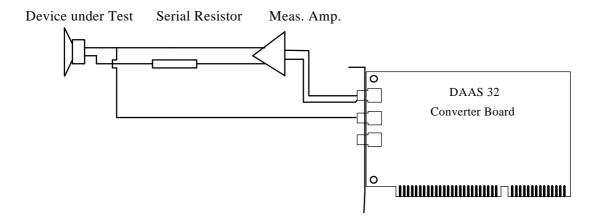
Measuring normally speakers use circuit one in conjunction with a serial resistor in the range  $150\Omega$ .
