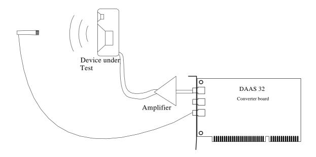
Position the microphone to the desired location and click or press the "In 2" button to select the acoustical input. Click or press the "Out" button and set the output attenuation to around 30-35 dB (the amplifier must not be over driven....clipping!). Click "Test level" to check the sound level. If the sound level is too high or too low this can be adjusted using the amplifiers volume control knob or the output attenuation.
