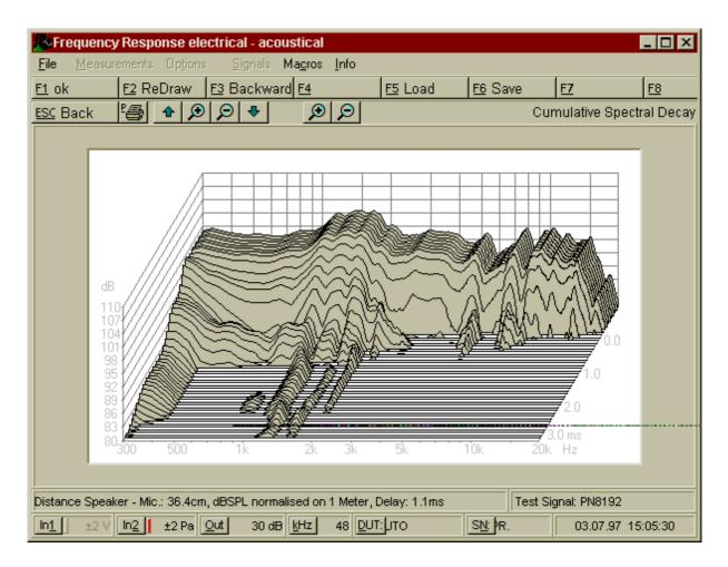
Here too the time axis can be altered with 'Zoom In t' and 'Zoom Out t'. However by using the zoom function all the curves are recalculated. The default setting for the time axis can be changed (see "Options").
