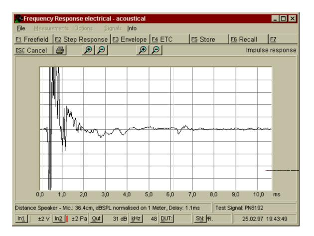
All signal parts to the left of the left marker (small vertical line) and to the right of the right marker line will be removed.
