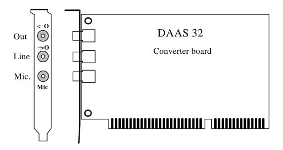
The DAAS<sup>®</sup>32 converter board has 2 inputs and one signal output. The microphone is connected to the "Mic" socket. Using the microphone supplied the maximum sound pressure is  $\pm 2$  Pa and  $\pm 8$  Pa.
