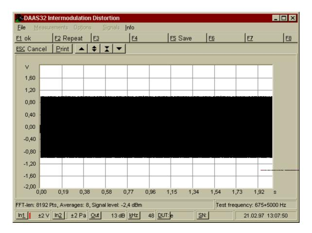
Pay attention that the tone with the higher frequency does not coincide with any harmonic wave of the tone with the lower frequency!
