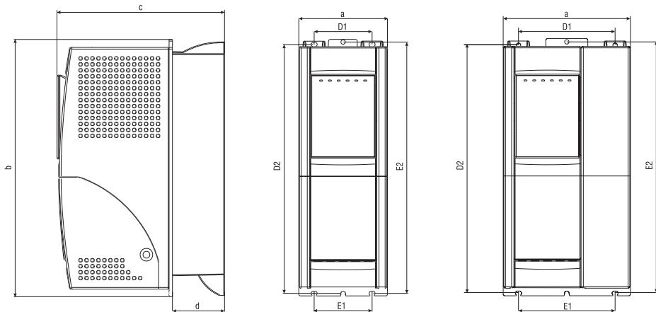
Figure 3.1.2: Mounting Methods (Sizes 1007 ... 3150)
