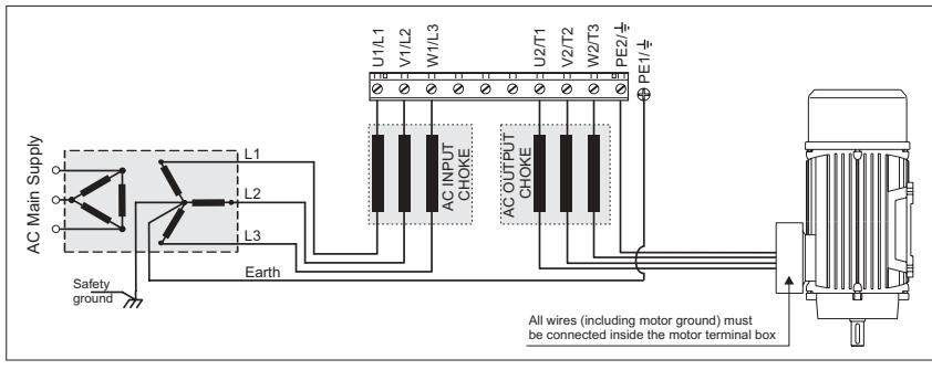
**Do not operate the Drive without the ground wire connected. The motor chassis should be grounded to earth through a ground lead separate from all other equipment ground leads to prevent noise coupling.**
