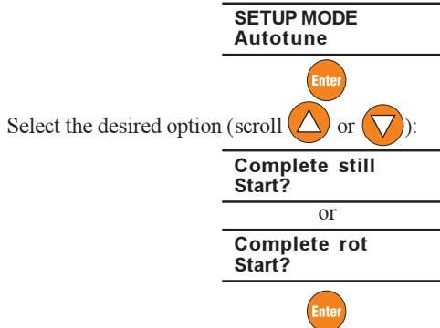
As standard example with motor and machine installed on system, **Complete still** are used. Connect terminal 12 (Enable) to terminal 19 (+24VDC) through relays or local switch, switch on the output contactors and leave the brake closed.
