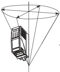
The maximum angle of inclination is 30°
