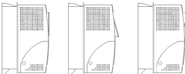
To allow a comfortable viewing angle, the keypad can be oriented on three different positions.
