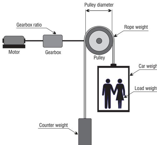
Press **Enter** to set Car weight (weight of the lift car), Counter weight, Load weight, Rope weight, Motor and Gearbox inertia parameter:
