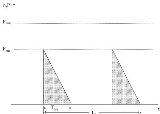
If one of the above mentioned rules is not respected, it is necessary to increase the tested power of the resistor, respecting the limit of the internal braking unit (reported intable 4.9.2.3), or an external BU if necessary.
