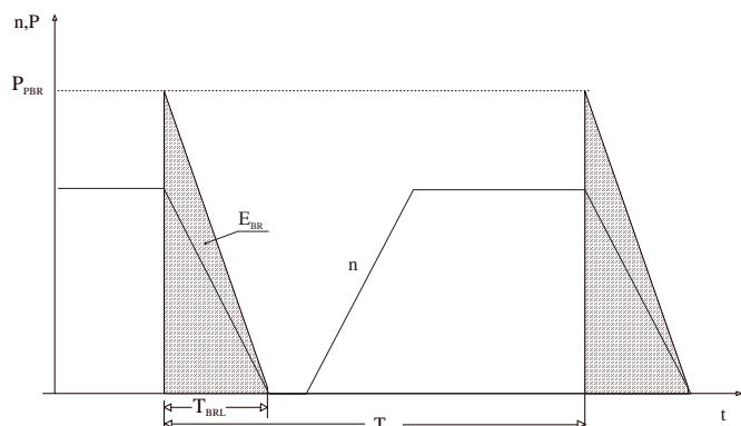
$T_{CL}$  Minimum cycle time in condition of limit operating cycle (braking power =  $P_{PBR}$  with typical triangular profile)
