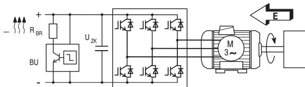
Drive sizes 1007 up to 3150 have, as standard configuration, an internal braking unit. Drive sizes 4220 up to 5550 can have an optional internal braking unit (see section 2.1.2 "Inverter type designation") factory mounted. All the standard AVy... drive can be equipped with an external braking unit (BU-32...) connected to the terminals C and D.
