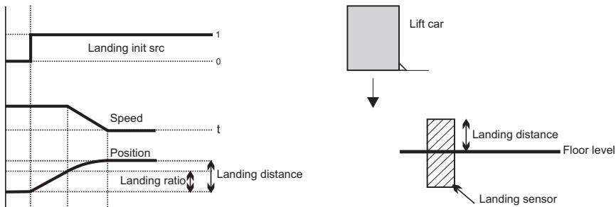
Landing sensor output can be interfaced to the drive through digital input which can become command to initialize landing control.
