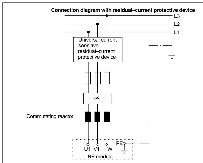
Fig. 2-12 Connection diagram, residual-current protective device
