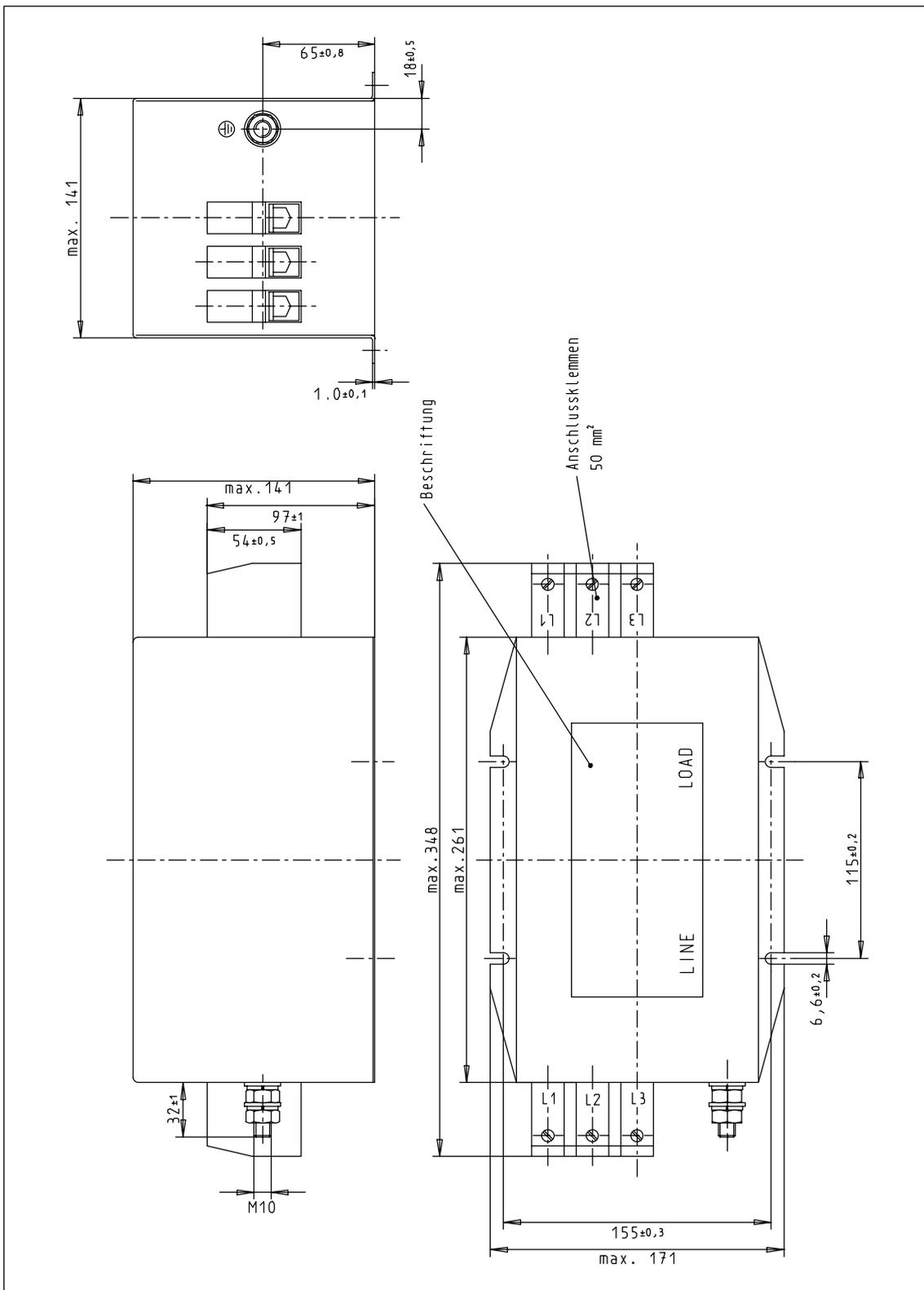
Fig. 13-9 Line filter 28 kW, 3GE.585455 TA aa, Sheet 2
