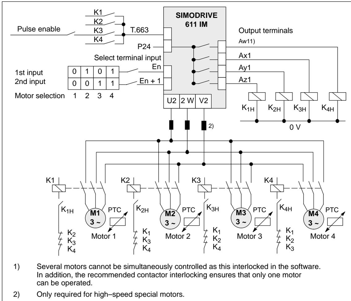
Fig. 9-30 Motor changeover at the SIMODRIVE 611 IM module
