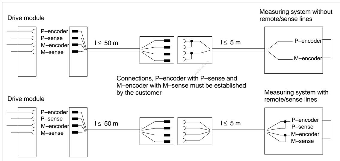
Fig. 3-5 Signal overview of the connections
