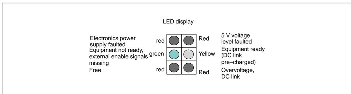
Fig. 6-9 LED display of the monitoring module
