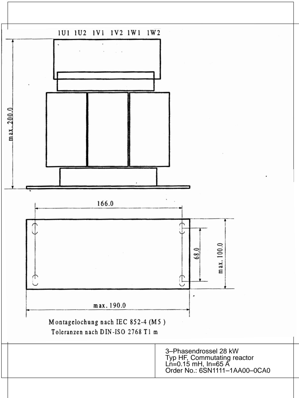
Fig. 13-20 3-phase reactor Typ HF, TA 585034, Sheet 2
