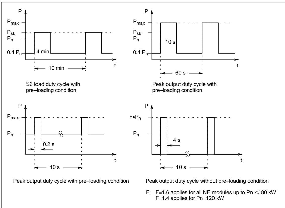
Fig. 6-5 Nominal load duty cycles for NE modules
