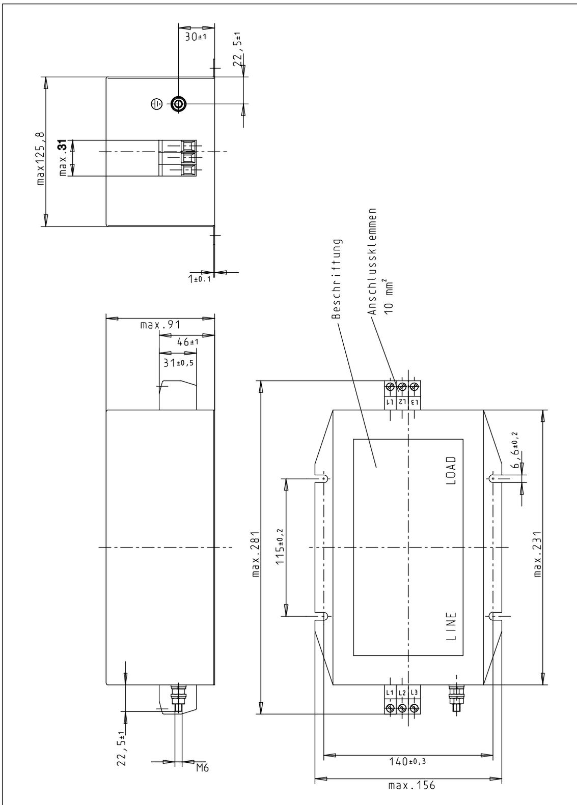
Fig. 13-8 Line filter 10 kW, 4GE.581785 TA ab, Sheet 2
