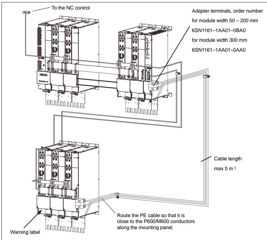
Fig. 10-3 Connection example, for a two-tier arrangement
