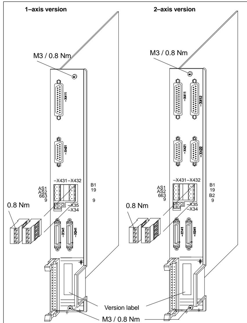
Fig. 5-7 Digital control with direct measuring system
