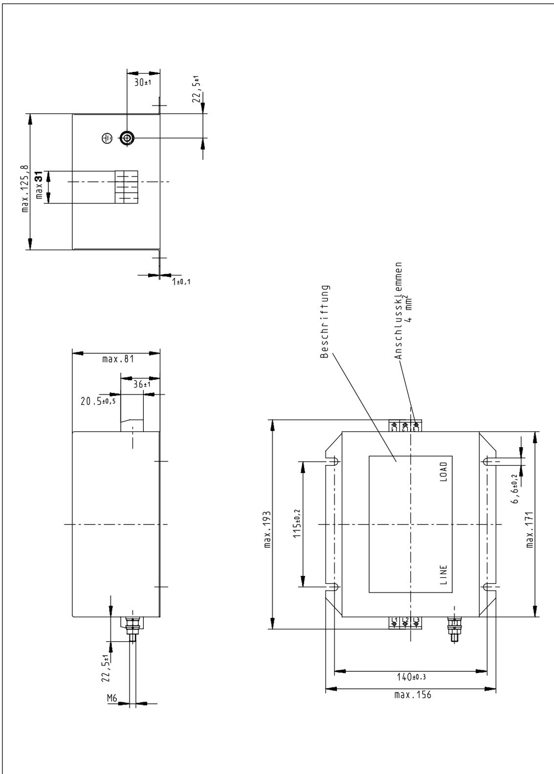
Fig. 13-7 Line filter 5 kW, 4GE.581793 TA ab, Sheet 1
