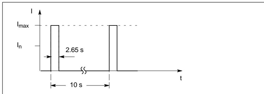
Fig. 4-5 Peak current – load duty cycle without pre-loading condition
