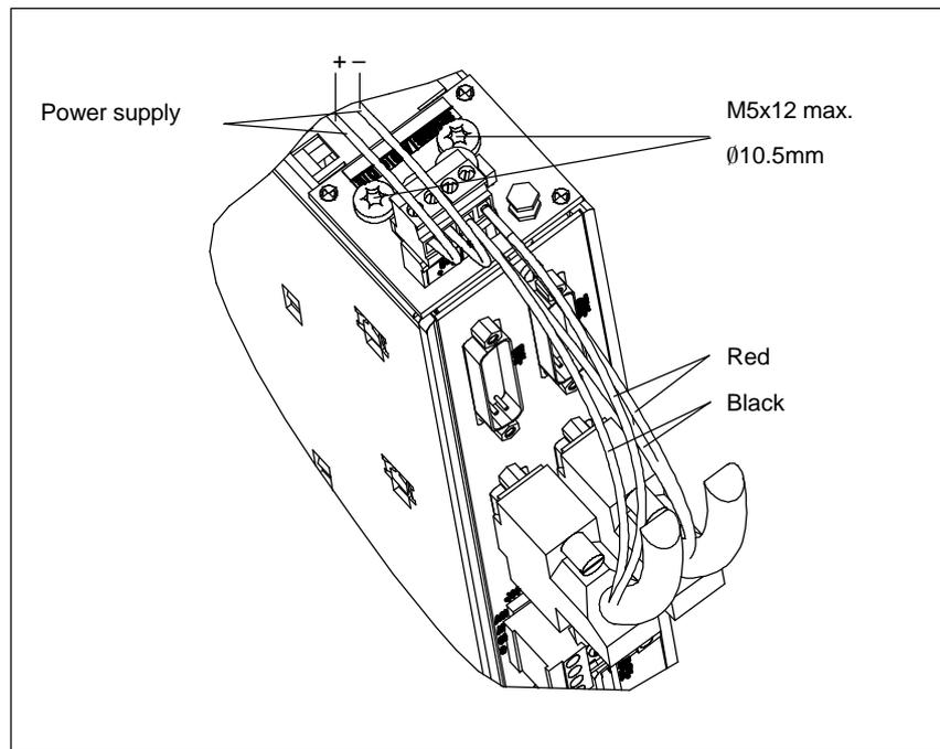
Fig. 3-9 Example of a connection at 6SN1118-0DG23-0AA1/-0DH23-0AA1
