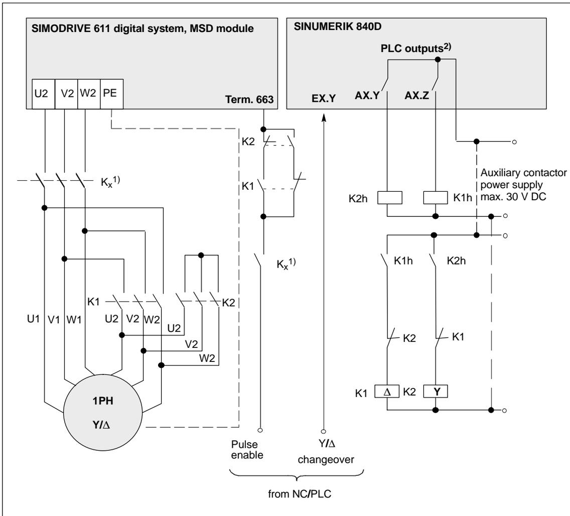
Fig. 9-28 Connection diagram for Y/ $\Delta$  changeover SIMODRIVE 611 digital
