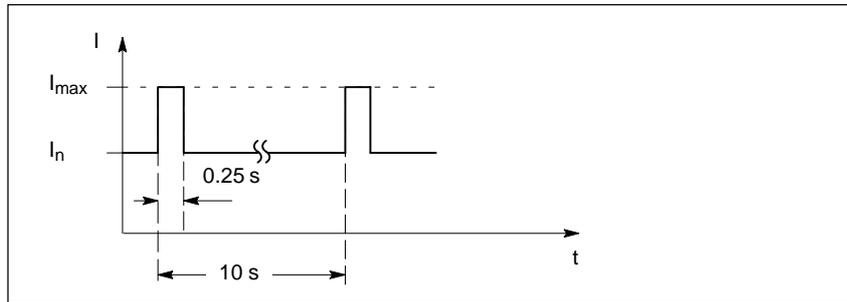
Fig. 4-4 Peak current – load duty cycle with pre-loading condition
