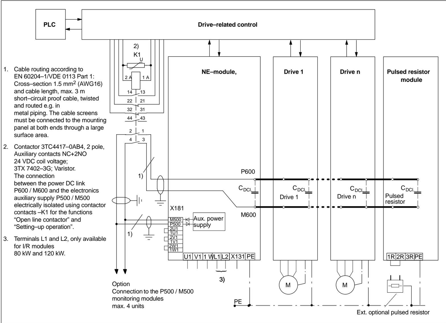
1. Cable routing according to EN 60204-1/VDE 0113 Part 1: Cross-section 1.5 mm<sup>2</sup> (AWG16) and cable length, max. 3 m short-circuit proof cable, twisted and routed e.g. in metal piping. The cable screens must be connected to the mounting panel at both ends through a large surface area.
