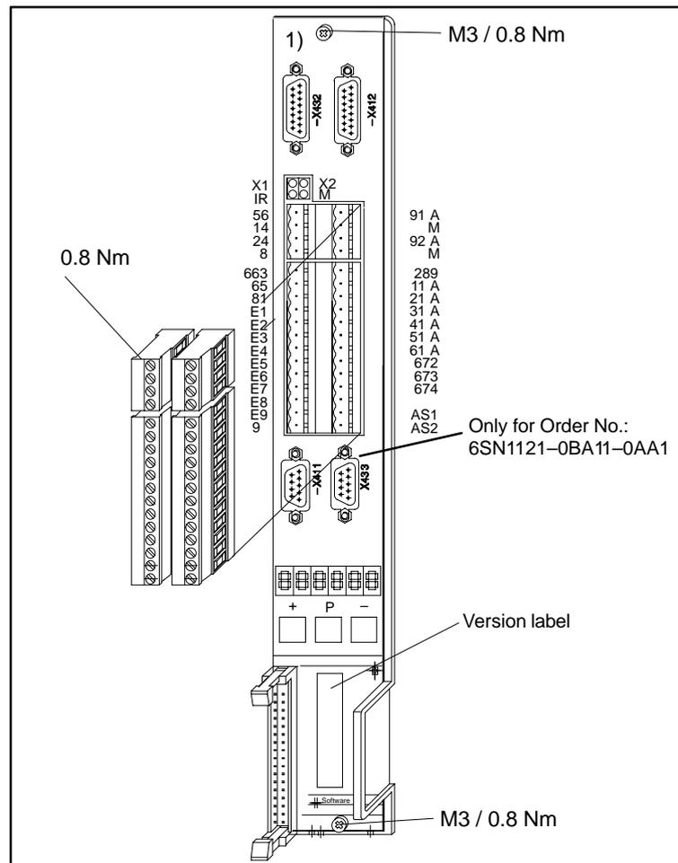
Fig. 5-5 Main spindle control with analog setpoint interface
