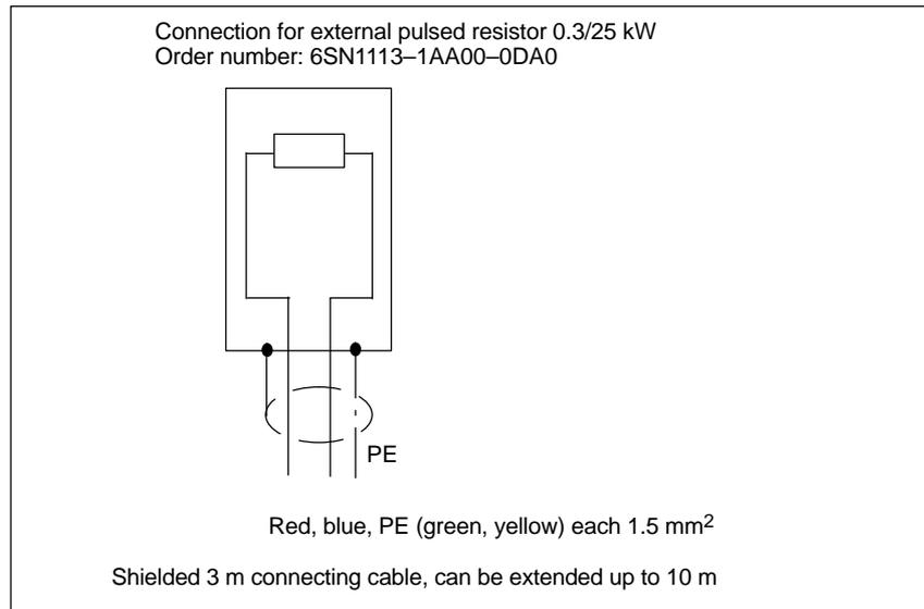
Fig. 6-14 Connection for external pulsed resistor 0.3/25 kW
