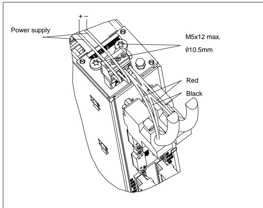
Fig. 3-10 Example of a connection at 6SN1115-0BA11-0AA1
