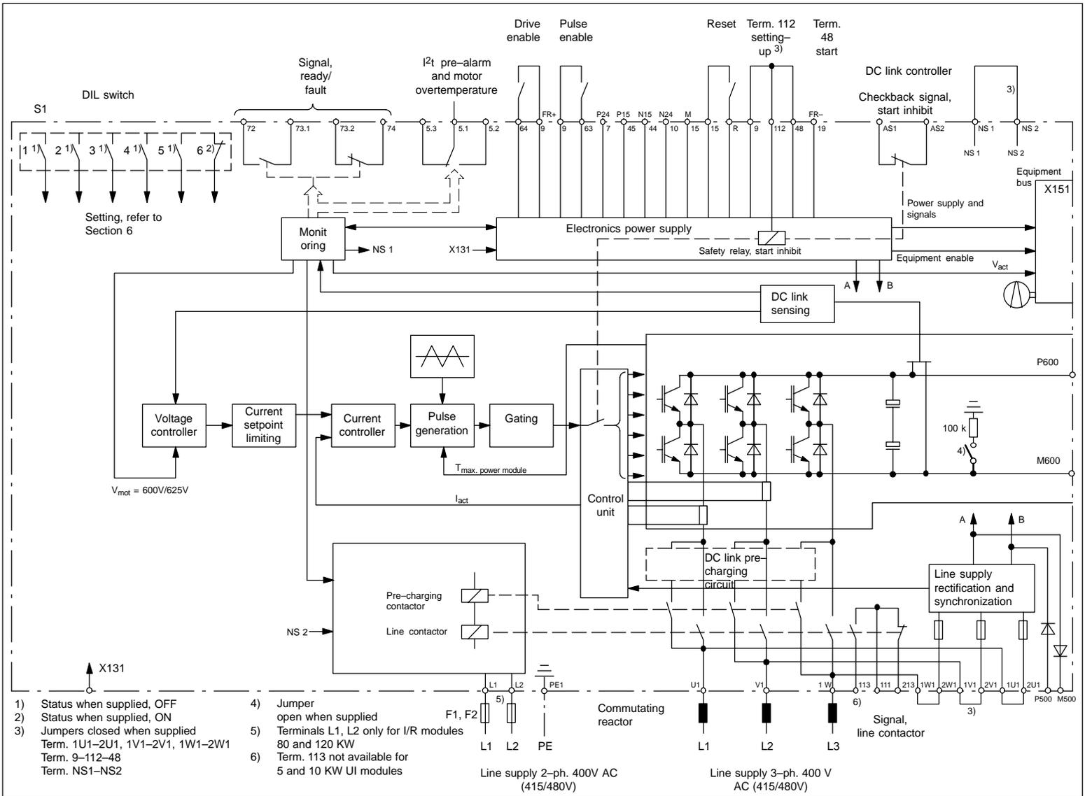
Fig. 6-3 Block diagram, line supply infeed module (I/R)
