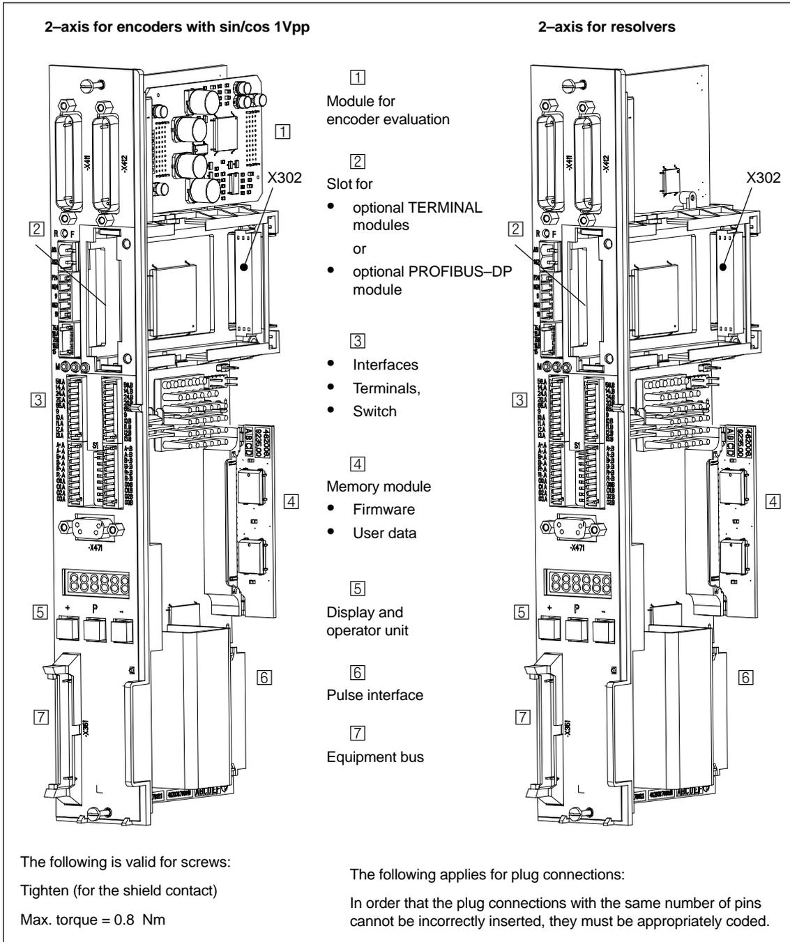
Fig. 5-8 Control modules for 2 axes
