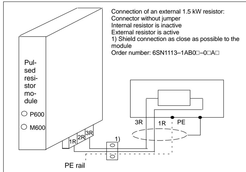
Fig. 6-17 Connecting an external 1.5 kW pulsed resistor
