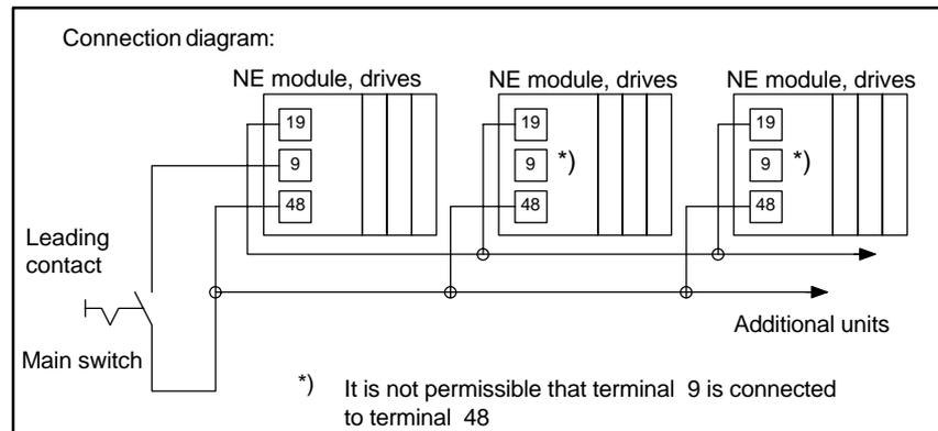
Fig. 9-3 Connection diagram of several NE modules at terminal 48
