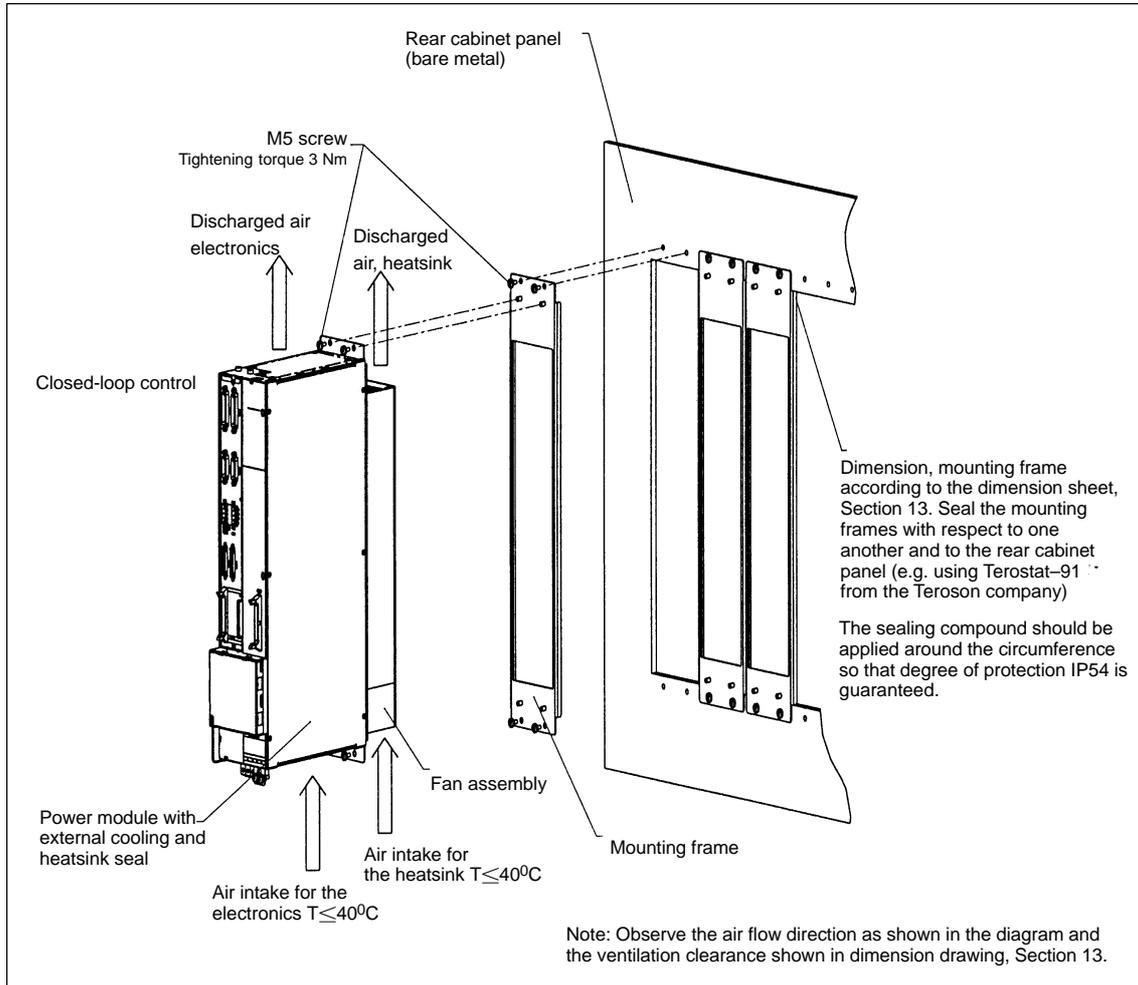
Fig. 2-7 Power module with inserted control module, external cooling
