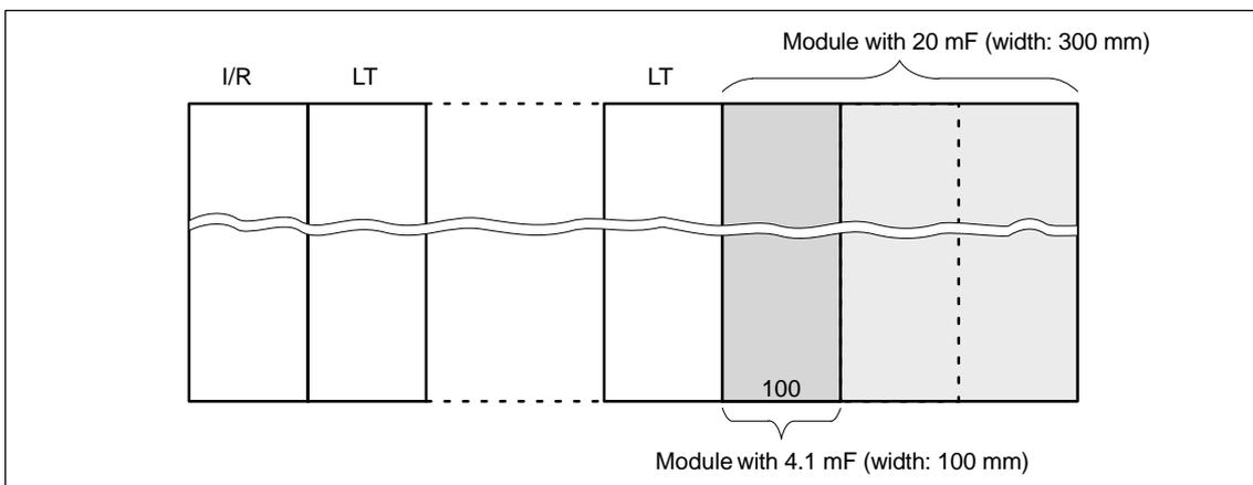
Fig. 6-12 Mounting location of the capacitor module
