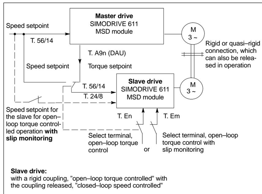
Fig. 9-25 Master/slave operation with an analog SIMODRIVE 611 system
