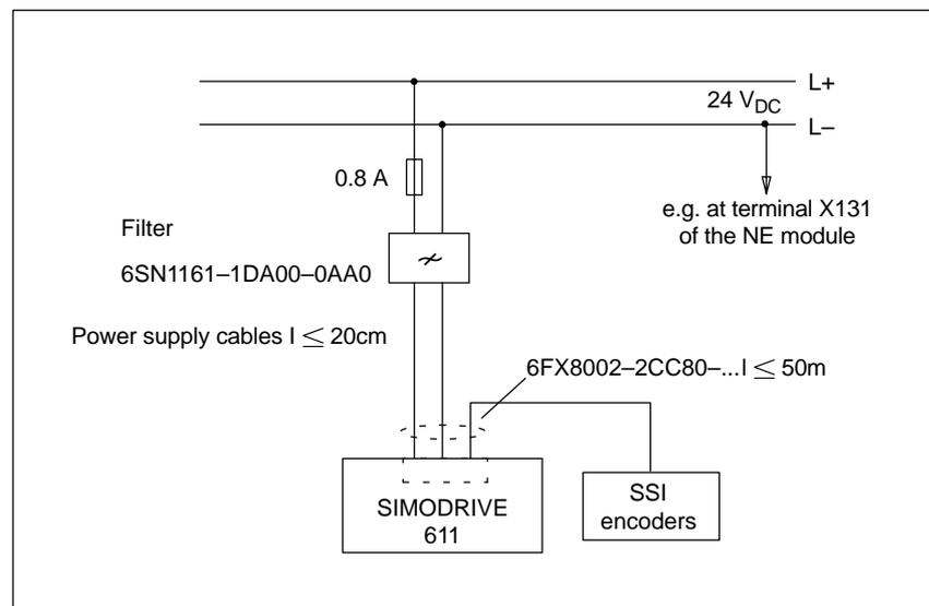
Fig. 3-8 Connecting SSI encoders to SIMODRIVE 611
