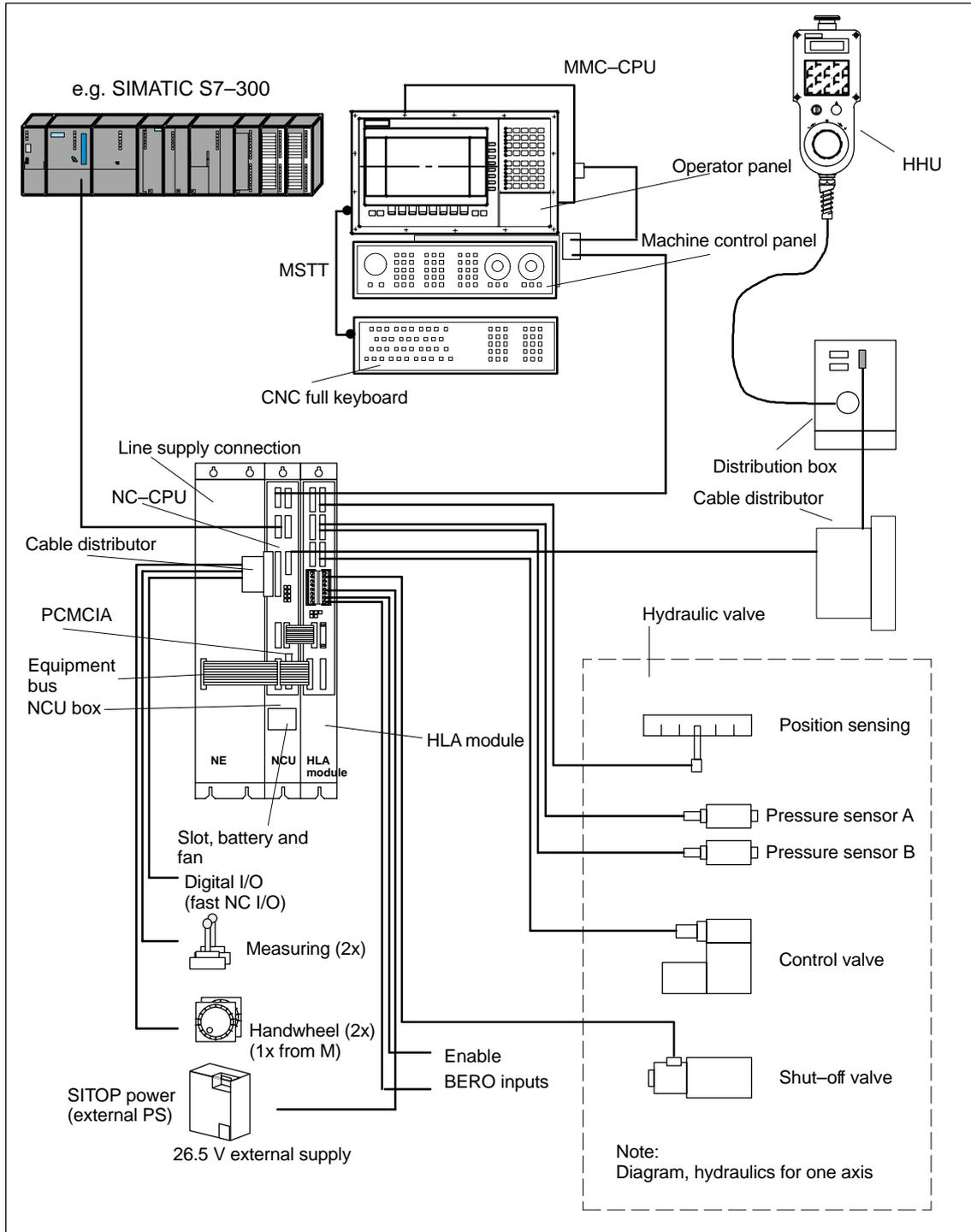
Fig. 5-13 System components
