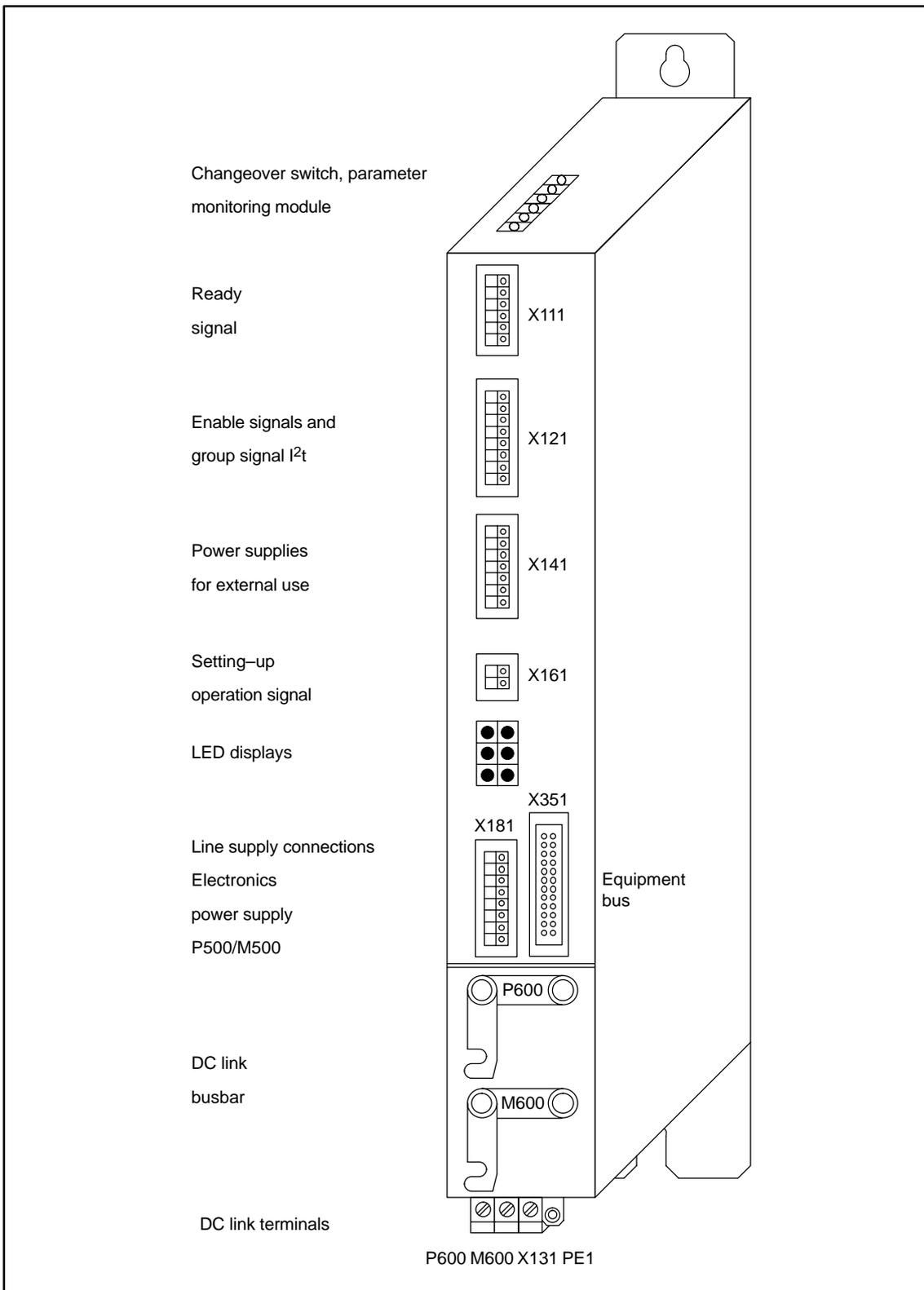
Fig. 6-8 Monitoring module 6SN1112-1AC01-0AA1
