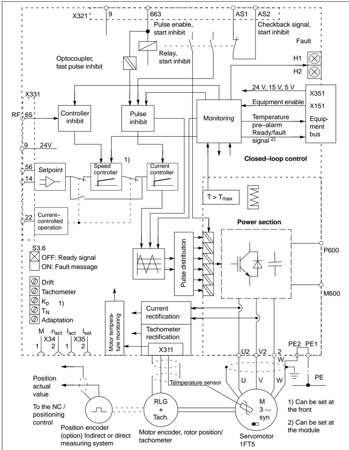
Fig. 9-8 Block diagram, FD module with standard interface
