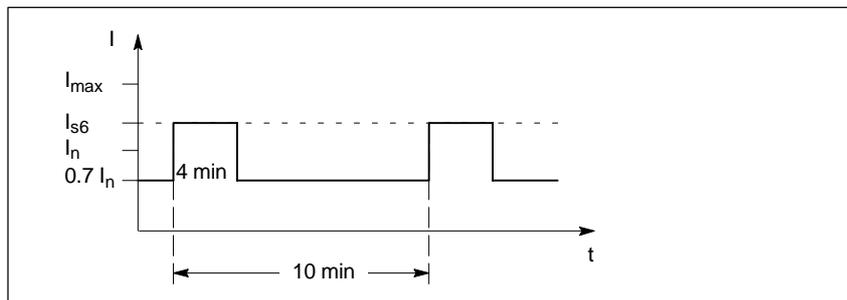
Fig. 4-6 S6 load duty cycle with pre-loading condition
