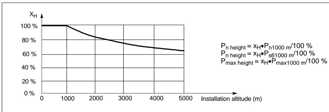
Fig. 6-6 De-rating depends on the installation altitude
