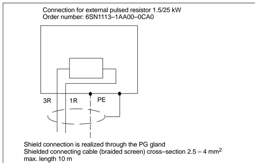
Fig. 6-15 Connection for external pulsed resistor 1.5/25 kW
