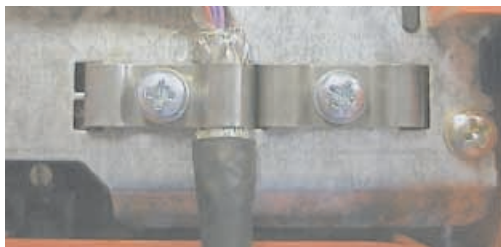
Fig. 17: Apply the shield to the electronics shield clamp of the inverter.
