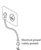
Grounded three-contact electrical outlet
