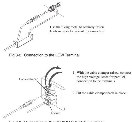
Fig.3-3 Connection to the IN HIGH VOLTAGE Terminal
