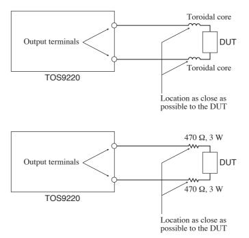
Fig.3-6 Reducing the Effects of Noise Generated by the Scanner
