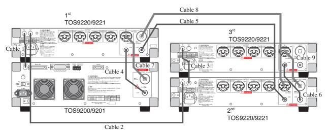
Fig.3-1 Connection of Three Scanners to the Tester Proper
