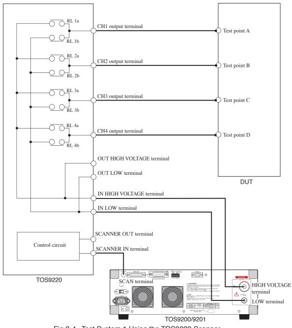
Fig.3-4 Test System 1 Using the TOS9220 Scanner
