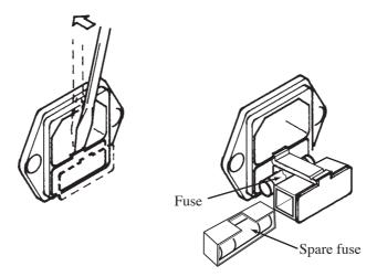
Fig.5-1 Removing the Fuse Holder
