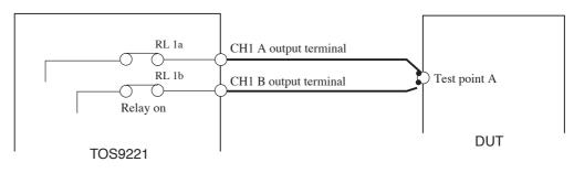
Fig.3-8 Connection Failure
