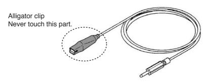
Fig.2-2 Supplied test leadwire
