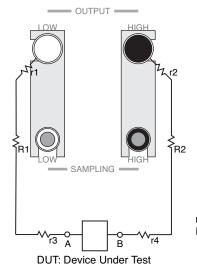
Install the short-circuit bars between the OUTPUT and SAMPLING terminals and connect the leads as shown in Fig. 2-5. The tester measures the total resistance value of contact resistance r1 to r4, resistance components R1 and R2 of the leads, and the resistance between A and B.
