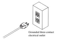
Connect the protective conductor terminal on the rear panel of the tester directly to ground.
