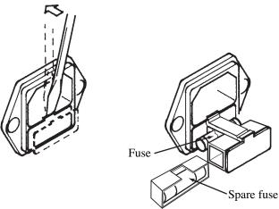
Fig. 7-1 Removing the Fuse Holder
