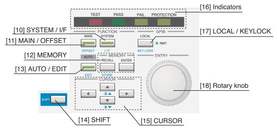
Fig. 3-2 Setup keys (example of TOS6210)
