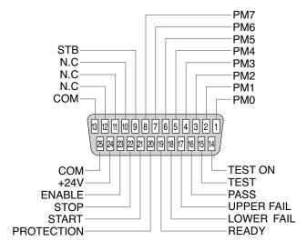
Fig. 5-3 SIGNAL I/O Pin Configuration
