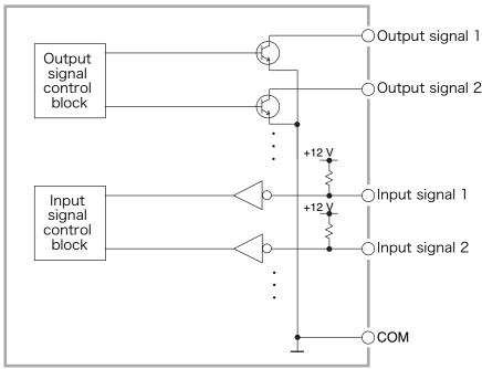
Fig. 5-4 Internal Configuration of the SIGNAL I/O Connector
