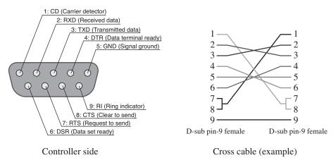
Fig.6-1 Pin-9 AT-type connector
