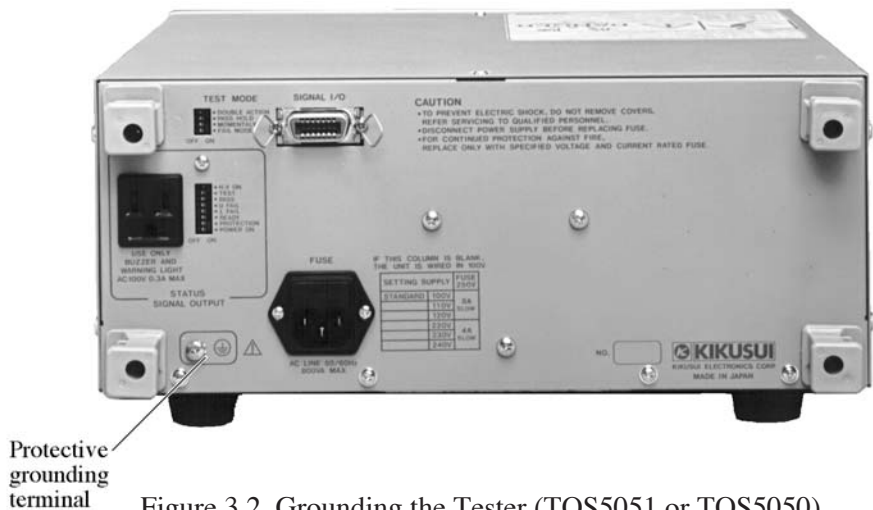
Figure 3.2 Grounding the Tester (TOS5051 or TOS5050)
