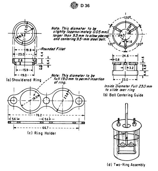
NOTE 1—All dimensions are in millimetres. FIG. 1 Shouldered Ring, Ball-Centering Guide, Ring Holder, and Assembly of Apparatus Showing Two Rings
