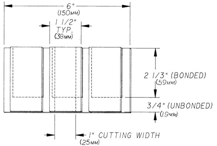
**FIG. 3 Slab Specimen**
