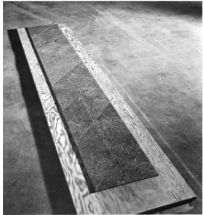
FIG. 7 Wood-Base Finish Floor Applied to Plywood with Tile Oriented so that Loaded Caster will Roll Across Corner
