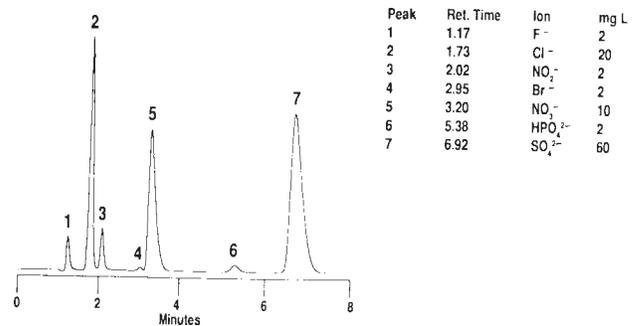
FIG. 1 Chromatogram Showing Separation Using the AS4A Column
