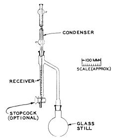
FIG. 1 Typical Assembly with Glass Still
