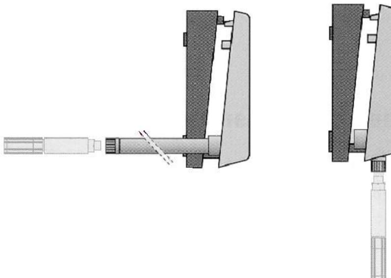
Once the base plate has been installed and wired, the electronics module can be inserted and secured with the screws provided. The transmitter is ready to operate.
