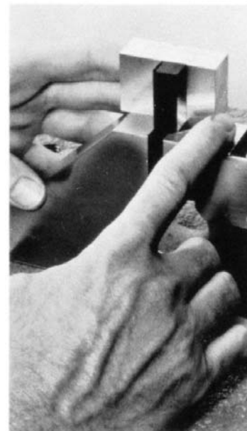
FIG. 4 Jig for Positioning Specimen for Clamping
