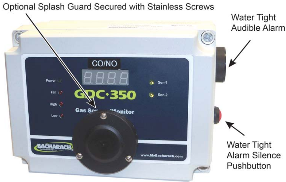
Figure 1-2. Water Tight GDC-350 Components
