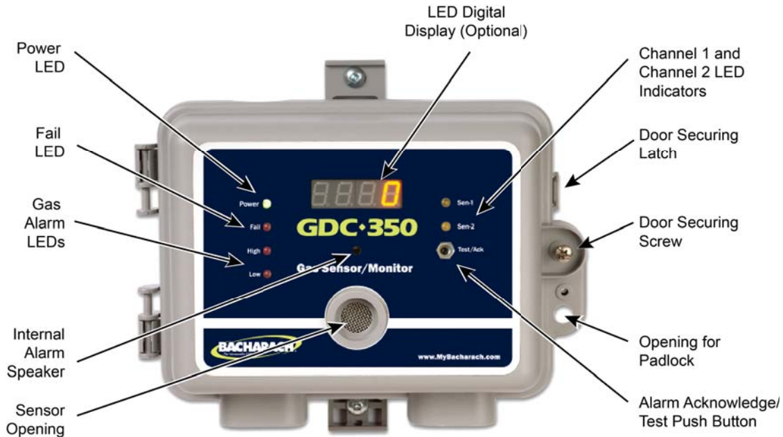
Figure 1-1. Standard GDC-350 Components
