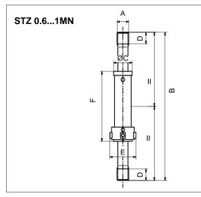
These special KD and STZ transducers are used to check out material testing machines and are designed in accordance to EN10002–3 or ISO 376. They are compressive force transducers and tensile force transducers that, because of their maximum overall height, are suitable for checking material testing machines according to ISO 7500-1.
