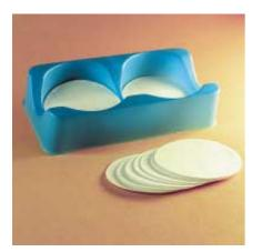
Hidex supplies glass fiber filter discs (dia. 47 mm, thickness 0.26 mm). They are ideal for wipe testing but find applications also in other fields, like air filtration (e.g. <sup>222</sup>Rn daughters) and binding assays in biosciences (cell harvesting, receptor-ligand binding etc.). The best performance is obtained with dried filters counted with MaxiLight cocktail.
