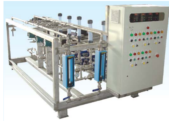
染料比例投加系统 Dye ratio dosing system
