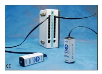
To provide the maximum in subject safety and isolation, use signal isolators to connect mains powered external equipment (i.e. chart recorders, oscilloscopes, etc.) to the MP System. Use the INISO isolator to connect to MP analog system inputs and the OUTISO isolator to connect to analog system outputs.
