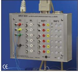
BS4 73-1790 Input Box Type 701/3 Signal Input for 12-Lead ECG and 6 Channels of MAP
