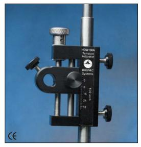
The HDW100A tension adjuster operates with the TSD105A and TSD125 series force transducers. The rugged design and stability of the mounting allow for fine position control. The position adjuster is located on the top for easy access and smooth operation. Vertical scales are provided for both metric and English units. The HDW100A slides directly onto vertical rod laboratory stands and force transducers are clamped into the unit horizontally.
