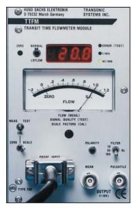
The Transit Time Flowmeter (TTFM) is an ultrasonic Transit Time flowmeter for animal research. It incorporates a complete 1-channel Transonic® ultrasonic transit time flowmeter. It can be used either with inline flow probes or perivascular probes from Transonic<sup>®</sup>, see page J7.
