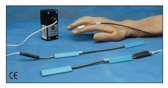
The TSD130 series goniometers measure limb angular movement. Goniometers attach to the body using TAPE2 medical adhesive tape. The units have a telescopic endblock that compensates for changes in distance between the two mounting points as the limb moves. The gauge mechanism allows for accurate measurement of polycentric joints. A DA100C is required for each output channel; accordingly, the twin-axis goniometers require two DA100C amplifiers to measure both axes simultaneously.
