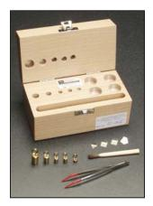
These gram calibration weights are precision weights use to calibrate preload on force transducers. The weights are made from polished brass. They are supplied in a wooden storage case with a pair of handling forceps and a cleaning brush. Nine weights are supplied. The 0.1, 0.2 and 0.5 gram size weights are flat metal pieces. The larger size weights have an integral hook. Class of accuracy M1 after OIML\*.
