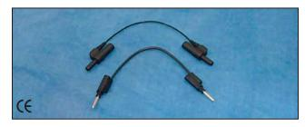
These jumper connectors (10 cm long) are used to create a common reference between Biopotential amplifier modules. Link one reference electrode to multiple amplifier inputs using one jumper connector per amplifier. Jumper connectors are required when connecting the same reference electrode lead to two or more amplifiers, as in multi-lead ECG or unipolar EEG measurements.
