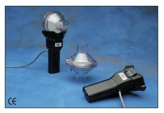
The TSD117 can be used to perform a variety of tests relating to air flow, lung volume and expired gas analysis. The transducer includes a removable head (RX117) for easy cleaning and sterilization. The TSD117 is intended for human use and is ideal for classroom situations. The TSD117 interfaces with the DA100C general-purpose transducer amplifier. All connections can be performed with AFT12 (22mm ID) tubing and AFT11 series couplers. See pages 1141 to 1143 for the AFT Series.
