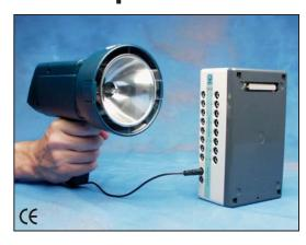
The TSD122 stroboscope connects directly to the UIM100C or STM100C module for single pass or averaging type visual evoked response applications. The stroboscope can be set up to either generate or respond to a TTL synchronizing signal for data acquisition. The TSD122 is battery-operated and will operate from zero to 12,000 flashes a minute. Cables are included for interfacing with the MP System.
