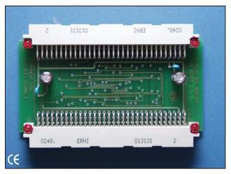
To mount backside modules on the front side of the system case
