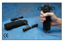
The TSD121C is an isometric dynamometer that measures a variety of gripping or pulling strengths for multiple muscle groups. The isometric design improves experiment repeatability and accuracy. Hand grip strength is easily recorded in pounds or kilograms force. Using the
