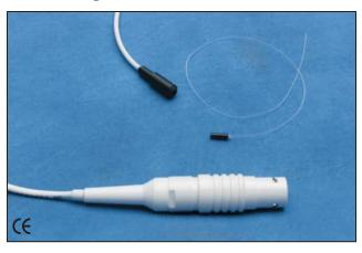
The TSD140 series disposable single fiber probes are designed for safe, continuous, invasive microvascular blood flow monitoring. The probes are thin flexible plastic fibers composed of a polymethyl methacrylate core and a tough fluorinated polymer cladding. All disposable probes are MRI compatible (no metal parts) and incorporate a coupling bead to interface with the TSD148 single fiber driver for connection to the LDF100C module.
