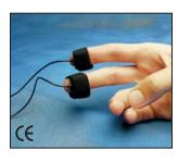
The TSD203 connects to the GSR100C amplifier for the purpose of skin conductance recording. Two Ag-AgCl, unpolarizable electrodes are mounted in individual, ergonomicallydesigned, polyurethane housings for improved contact. The electrodes are attached to the
