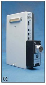
The DA100C is a very low noise and drift differential bridge amplifier that will operate with a wide variety of transducers, including: pressure, force, strain, displacement, thermocouplers, piezo sensors, light sensors, microphones and nearly any other active or passive sensor or transducer. The DA100C provides variable gain settings, offset control for baseline zeroing and adjustable voltage references for activating passive transducers (see pages I121 to I132).
