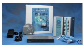
The new MP150 offers Ethernet-ready data acquisition and analysis. Record multiple channels with differing sample rates. Record at speeds up to 400kHz (aggregate). Place one or more MP150 Systems in a local area network (LAN). Use any PC in the LAN to record from any MP150 System in the LAN. Includes:
