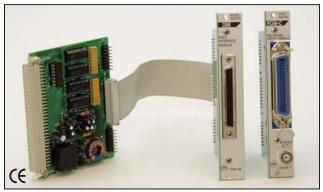
ROM DL board with DIM or ROM C. DIM is used for A/D board connection.
