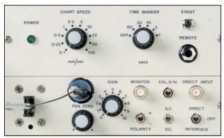
These oscillographs are designed around a pen amplifier module which contains the circuits to power the pen and operate the various amplifier interface modules on the following pages. The oscillographs are supplied with 2 or 4 factory-installed pen amplifier modules with either curvilinear or rectilinear writing.
