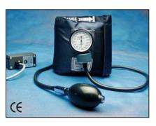
The TSD120 can measure systolic and diastolic blood pressure by the oscillometric or auscultatory (Korotkoff sounds) technique. The TSD120 includes an adjustable cuff (standard adult cuff: RX120D), pump bulb, pressure gauge and pressure transducer. The pressure transducer is attached to the cuff and connects to the DA100C
