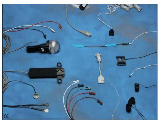
Smart Sensor (SS) electrodes and transducers connect to the TEL100M-C amplifier/transmitter. Any Smart Sensor electrode or transducer can be plugged into any TEL100M-C input. The following SS series transducers connect to the TEL100C system. The transduc-
