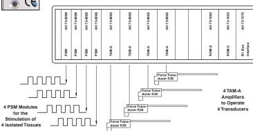
Sample PLUGSYS Setup: PLUGSYS Equipment for Stimulated Isolated Tissues Module
