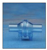
The TSD127 can perform a variety of pulmonary measurements relating to air flow, lung volume and expired gas analysis. The transducer includes a detachable flow head (RX127) for easy cleaning and sterilization. The TSD127 is intended for animal use and consists of a low flow, pneumotach air flow head (RX127) coupled to a precision, highly sensitive, differential pressure transducer (TSD160A). The TSD127 will connect directly to a breathing circuit or plethysmogram chamber.
