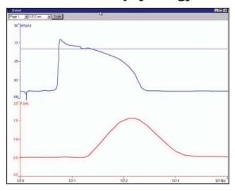
Two channel data acquisition software for electrophysiologic studies on papillary muscles or purkinje fibres in a horizontal tissue bath (e.g. HSE Steiert papillary bath).
