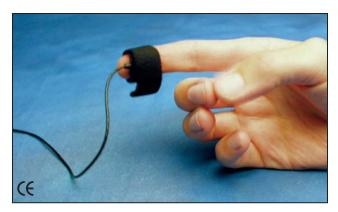
This transducer operates with the PPG100C amplifier to record the pulse pressure waveform. The TSD200 consists of a matched infrared emitter and photo diode, which transmits changes in infrared reflectance resulting from varying blood flow. The ergonomic housing design improves contact with the subject and helps reduce motion artifact. The TSD200 is primarily designed for finger attachment, but can be taped to other body locations. The TSD200 comes with a shielded 3-meter cable.
