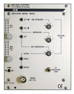
The Ventilation Control Module VCM has been developed especially for producing a negative pressure at a respiratory rhythm as required for operating an isolated perfused rabbits, rats, guineapigs, or mouse lung.
