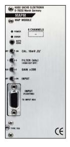
The MAP module Type 703 is for capturing and amplifying monophasic action potentials (MAPs) in the PLUGSYS system. It has to be connected to special MAP electrodes. This module incorporates isolated input amplifiers in order to avoid hum interference. In this way the inputs are isolated electrically from the output circuits and from the housing.
