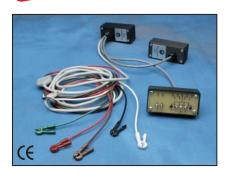
The TSD155C multilead ECG cable is used for performing a standard 12-lead ECG recording using only 3 ECG100C amplifiers. TSD155C permits simultaneous recording of Leads I, II, III, aVR, aVL,
