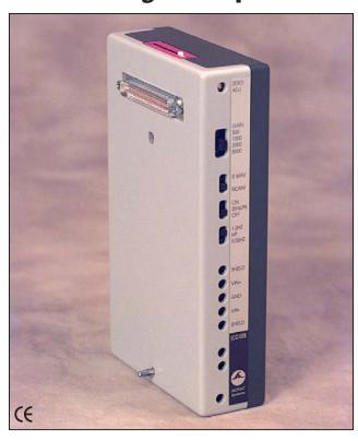
The ECG100C records electrical activity generated by the heart and will reliably record ECG from humans, animals and isolated organ preparations. The amplifier output can be switched between normal ECG output and R-wave detection. The R-wave mode outputs a smoothed pulse with the occurrence of each R-wave. The exact timing of the R-wave is detected even under conditions of extreme signal artifact. The amplifier also includes a user-switchable baseline stabilizer.
