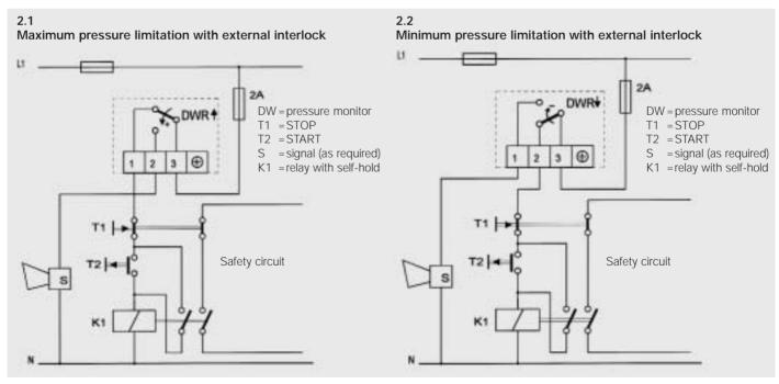
When the interlock circuit shown above is used, the requirements in accordance with DIN 57 116/VDE 0116 are fulfilled if the electrical equipment such as contactors or relays of the external interlock circuit correspond to VDE 0660 or VDE 0435 respectively.
