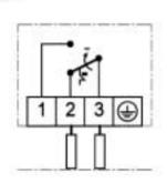
A pressure monitor (microswitch with automatic reset) can also be used as limiter if an electrical interlock in connected in series. In pressure limitation in steam and hot water boilers, the external interlock is permissible only if it is ensured that the pressure monitor is of "special construction".
