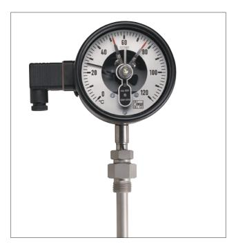
A glycerine filled indicator version is available as an option for service at measuring points exposed to strong vibrations. The fill dampens the measuring system when exposed to mechanical vibrations and thus enables steady indication; it also provides good lubrication for moving parts.
