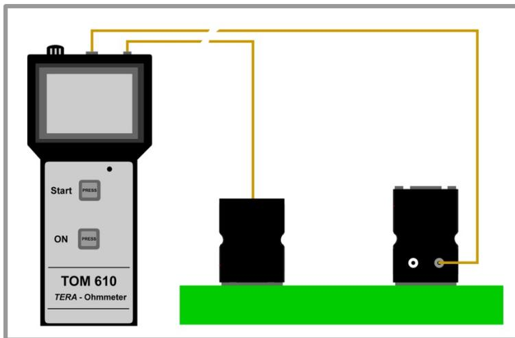
TOM610 测试表+REM002 电极+REM003 电极
